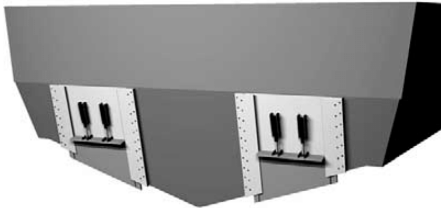
Figure 1.1: Two transom interceptors mounted to the stern of a vessel. These devices are lowered into the oncoming flow, generating lift by creating a stagnation point. Note the sharp angle between the stern and keel instead of being rounded. Modified image from Rijkens et al. (2011).
