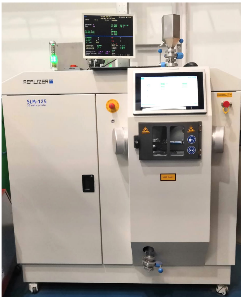
Figure 37: Selective laser melting set up
