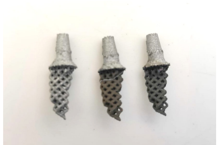
Figure 61: Implant non treated, PEO treated, PEO+silver treated
