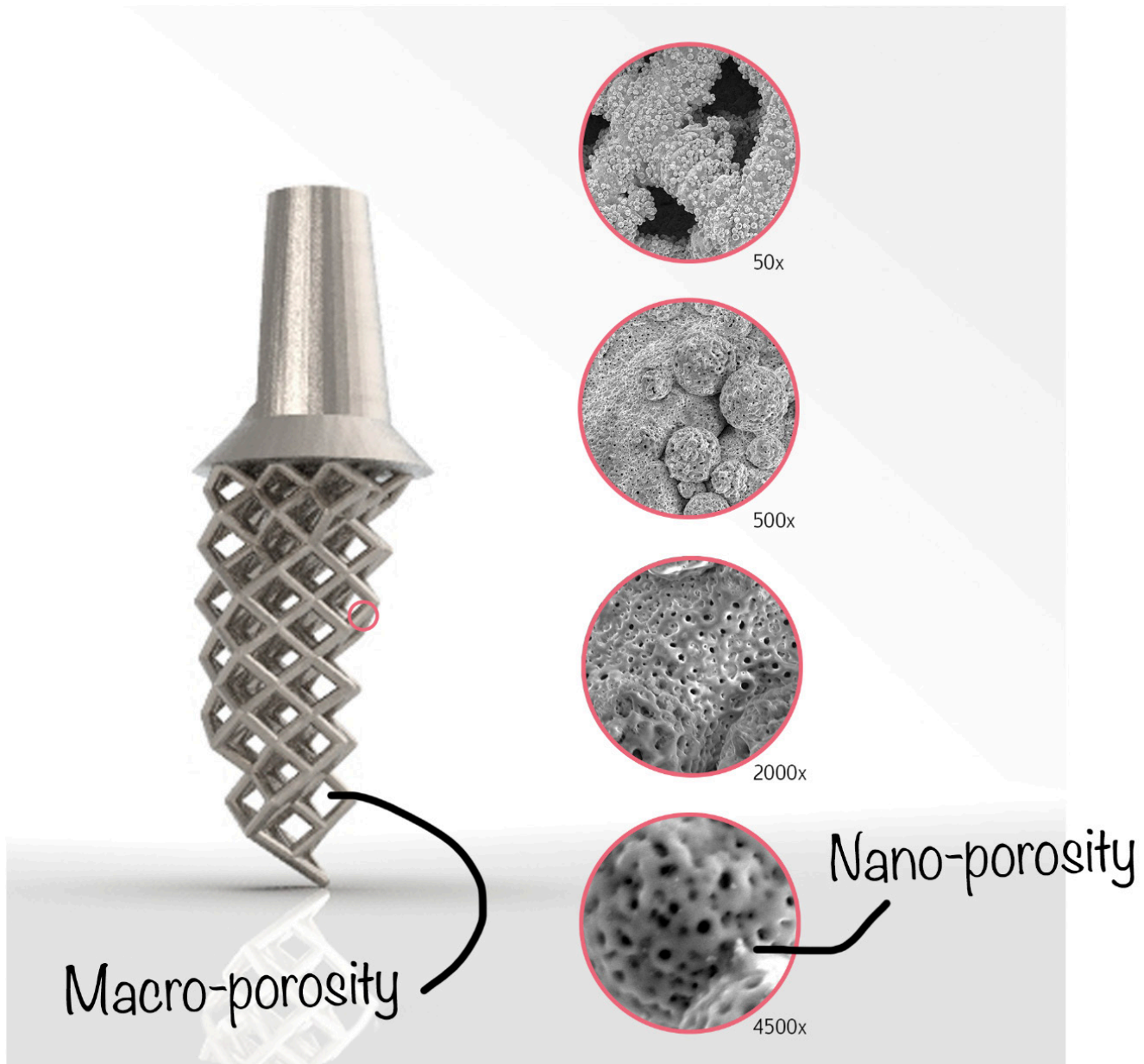
Figure 42: Design concept with its macro-porosity (lattice structure) and its nano-porosity
