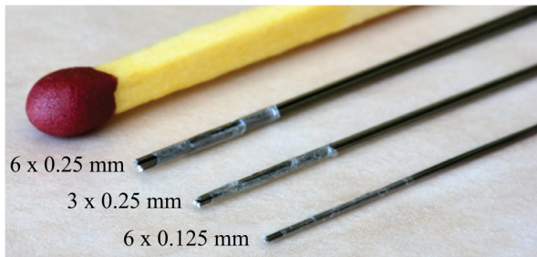
Figure 1.2: The needle systems of the designs by Scali et al. [15]. The designs feature different needle amounts and thicknesses and are held together by PET tubes.
