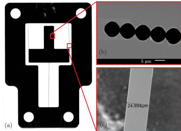
Fig. 9. Micrographs of a balanced stage. (a) A picture of a balanced stage. It can be observed it is buckled in the mode from Fig. 5b. (b) A SEM image of the markers used to align the microforce sensing probe with the center of compliance, see Fig. 4b. In figure (c) a typical SEM image used for measuring the beam width is shown.
