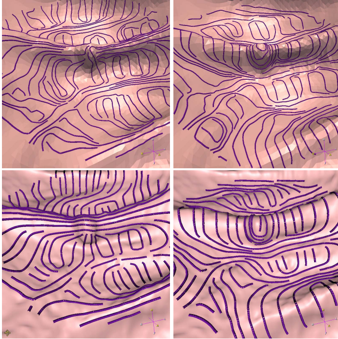
Figure 4.9: Comparison of curvature streamline appearance on the triangle mesh and the iso-surface of a medical 3D volume data: Left two show streamlines of minimum curvature, right two show streamlines of maximum curvature.
