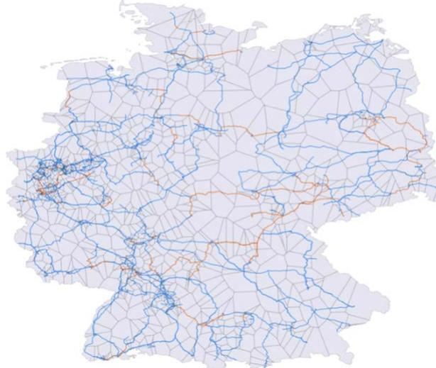
**Figure 5.20:** *Voronoi Regions and Transmission Corridors for Germany. In Red the simulated above 80% loaded (N-1 overloaded) lines on 01:00:00 1/1/2010.*
