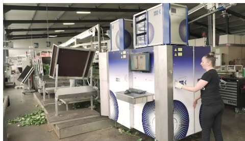
Figure Appendix B1 IRISS installed on sorting machine
