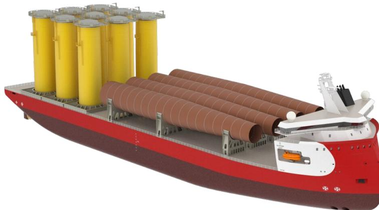
Figure 1.1: A rendered image of a heavy transport vessel (HTV)
