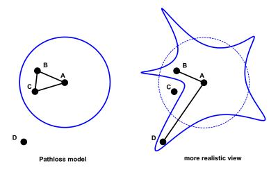
Figure 3.8: Schematic view showing the nondeterministic nature of radio links where in reality short distance links may not exist while longer distance links do.
