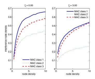
Figure 8.3: Density of interfering nodes found by simulations for MAC classes 1, 2 and 3. Left subplot:  $0.5 \le \rho \le 10$  and  $\xi = 0$ , right subplot:  $0.5 \le \rho \le 10$  and  $\xi = 3$ .
