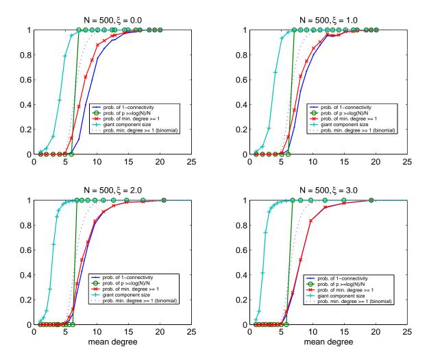
Figure 6.1: Simulated results for different values of  $\xi$  showing: the probability of 1-connectivity, the probability of p exceeding the log(N)/N threshold, the probability of the minimum node degree being more than or equal to one, and the giant component size as fraction of the total number of nodes. For comparison reasons, we have drawn on each graph the probability of minimum degree being more than or equal to one for a binomial degree distribution.
