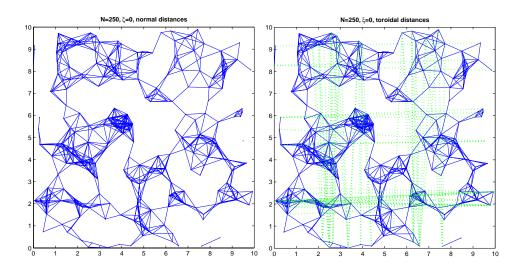
Figure 4.3: Links between nodes in an rectangular area (figure on the left), and new links that appear when toroidal distances are considered (figure on the right).
