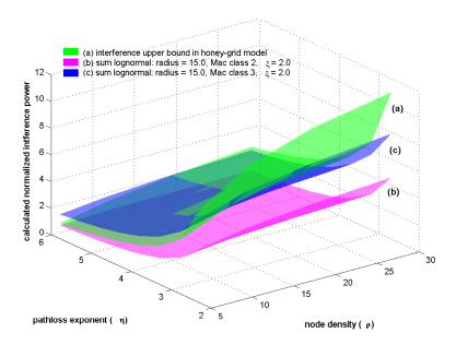
Figure 9.7: Comparison of interference upper bound (9.6) with interference calculated using the lognormal summation method. In this plot we have taken radio signal power fluctuations into account ( $\xi = 2$ ).
