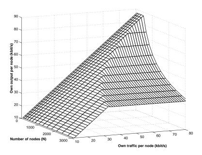
Figure 10.10: Portion of the throughput per node assigned to a node's own traffic. All values and assumptions are the same as in Figure 10.9.
