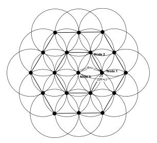
Figure 9.1: Constellation of interfering nodes around node 0 when we arrange interfering nodes in positions to obtain the maximum number of interferers.
