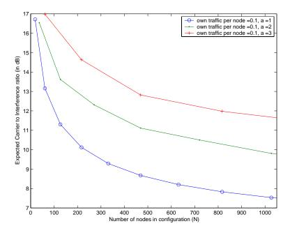
Figure 10.5: Expected value of C/I for a node in the center of a honey-grid structure for different values of a node's reach, a. In all cases the pathloss exponent is 2.4, the node's own traffic rate is 0.1 packets per time-slot and the processing gain is 10.4 dB.
