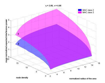
Figure 8.9: Expected mean interference power as function of the network node density and area size for  $\eta = 3.0$  and  $\sigma = 4.0$ .
