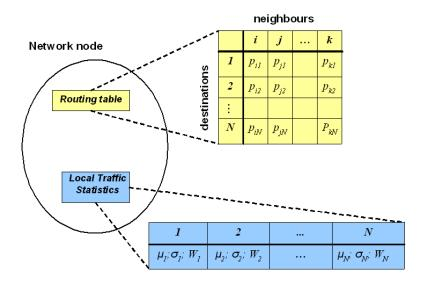
Figure B.2: Routing table and local traffic statistics in ant-routing...
