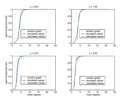
Figure 6.7: Simulated and calculated values for the giant component size in wireless ad-hoc networks for different values of  $\xi$ .
