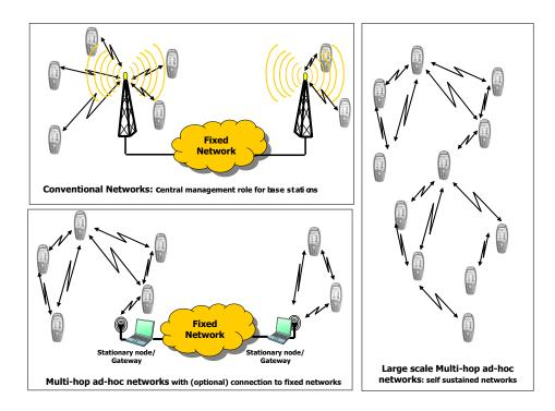
Figure 1.1: Comparison of wireless cellular and wireless ad-hoc network concepts.
