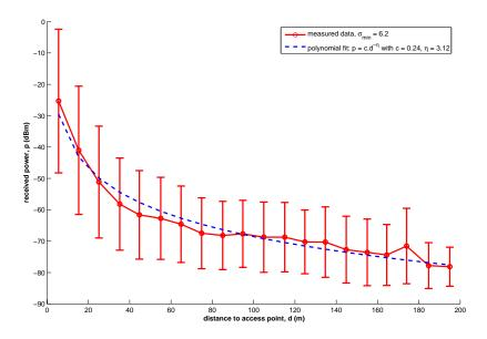
Figure 3.12: Power as function of the distance to access points. Error bars show the standard deviation of measured data.
