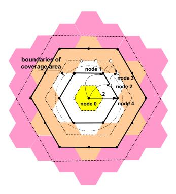
Figure 9.4: Relay rings and relay nodes in a honey-grid. Thick lines show relay rings. Dark filled circles are relay nodes. Hollow circles are other nodes in the network.
