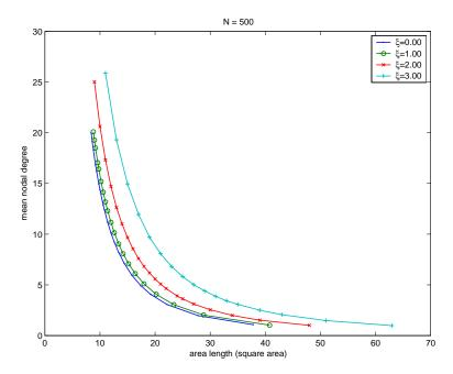
Figure 6.4: Mean node degree for 500 nodes uniformly distributed over areas of different sizes for different values of  $\xi$ .
