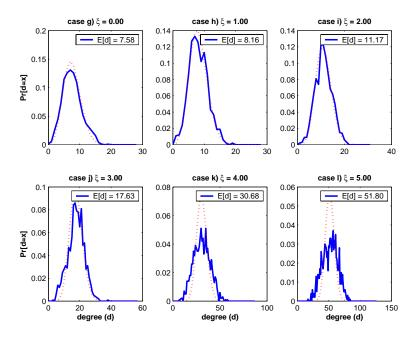
Figure 4.5: Degree distribution found through simulation for different values of  $\xi$ , compared with a binomial distribution having the same mean value. Service area in all cases is  $20 \times 20$  and N = 1000.
