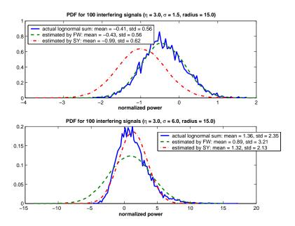
Figure 8.5: Test of the FW and SY interference power estimation for lognormal distributed interference signals coming from known distances spread over a circular area.
