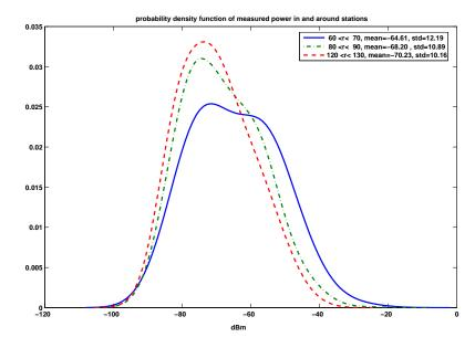
Figure 3.13: Probability density function for some range of measured data. Lines in this figure show the contour of the PDF's.
