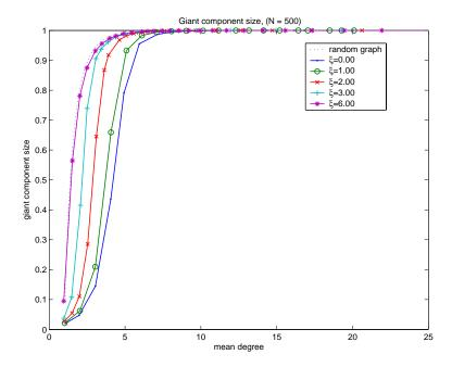
Figure 6.6: Comparison of the giant component size in a random graph with the values found for wireless ad-hoc networks.
