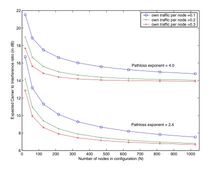
Figure 10.4: Expected value of C/I for a node in the center of a honey-grid structure for different values of a node's own traffic,  $\lambda$ . In all cases the node's reach, a, is 1 and the processing gain is 10.4 dB.
