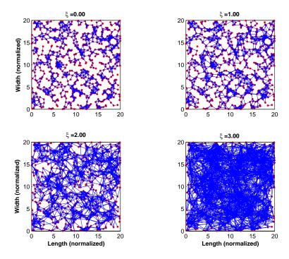
Figure 5.1: Nodes and links in an ad-hoc network for different values of  $\xi$ . In all subplots N = 1000, and service area is  $20 \times 20$ .
