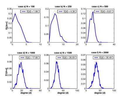
Figure 4.4: Degree distribution found through simulation for different values of N, compared with a binomial distribution having the same mean value. Service area in all cases is  $20 \times 20$  and  $\xi = 3$ .
