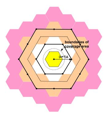
Figure 9.5: Honey-grid with interfering rings (thick lines) for a = 1.
