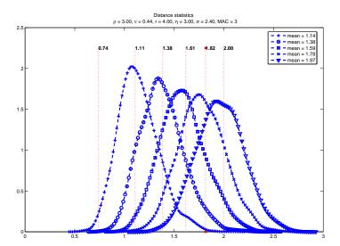
Figure 8.6: Calculated distances of interfering nodes to the center node and the simulated probability density function of the distance of interfering nodes to the center node in an ad-hoc network with r = 4,  $\rho = 3$ ,  $\eta = 3$ ,  $\sigma = 2.4$  and MAC class 3.
