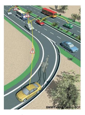
Figure 1.2: BMW talking cars for local hazard warning: a working example of a commercial application of ad-hoc networks. The car's on-board computer uses data coming from the brakes and ABS monitoring systems to decide whether and when to transmit a hazard warning to other vehicles in its vicinity. This hazard waning can then be relayed up to a predefined number of hops to other cars.
