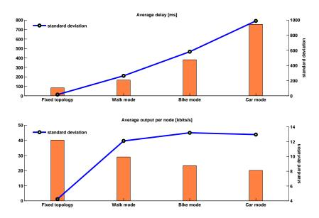
Figure B.3: A set of simulation results found using ant-net simulator. The walk mode, bike mode and car mode correspond to node speeds of, respectively, 5 km/h, 15 km/h and 75 km/h.
