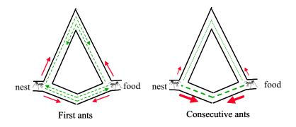
Figure B.1: The principle of ant-routing.
