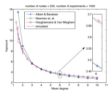
Figure 3.3: Comparison of three hopcount formulas with simulated values for a random graph of 500 nodes. Simulation results are average values for 1000 experiments, with standard deviation shown as error bars. For better visibility, we have blown up the section around the mean degree of 6.
