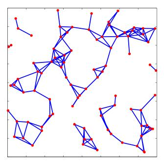
Figure 3.1: Snapshot of an ad-hoc network. In this graph, dots represent nodes forming the network and lines indicate links between nodes. Links are assumed to be established over wireless channels.
