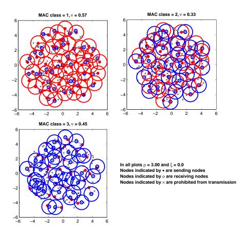
Figure 8.1: The working of MAC classes 1, 2 and 3 on randomly distributed nodes with the density of 3 nodes per normalized area of  $1 \times 1$  in a circular service area of normalized radius 5 with  $\xi = 0$ .
