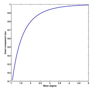
Figure 3.4: Growth of the giant component size as function of the mean nodal degree in a random graph.
