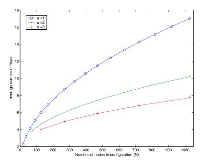
Figure 10.3: Mean value of the hopcount in a honey-grid structure for different number of node (N) and different values of a (reach of a node).
