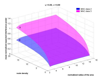
Figure 8.10: Expected mean interference power as function of the network node density and area size for  $\eta = 6.0$  and  $\sigma = 8.0$ .
