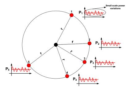
Figure 3.7: Simplified indication of small scale and medium scale ( $p_i$ 's) power fluctuations. The mean of many  $p_i$  values, corresponds to the large scale area mean power at distance r.
