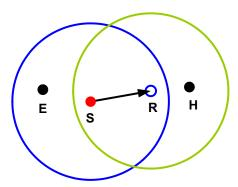
Figure 7.1: Schematic view of Sending, Receiving, Hidden and Exposed nodes (terminals) in packet radio communication networks.
