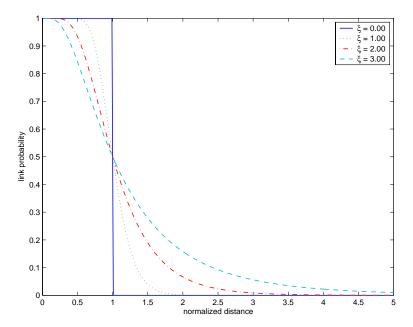
Figure 3.10: Link probability in lognormal geometric random graph model for different  $\xi$  values. In the case  $\xi = 0$  the lognormal model reduces to the pathloss model with circular coverage per node.
