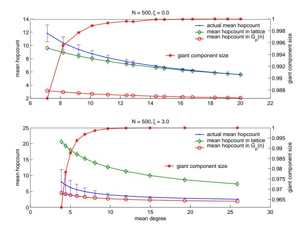
Figure 6.3: Simulated results showing the mean hopcount as function of the mean degree for different values of  $\xi$  in ad-hoc networks in comparison to the mean hopcount in lattice networks and random graphs. Error bars on the line for actual hopcount indicate the standard deviation of the simulated hopcount.
