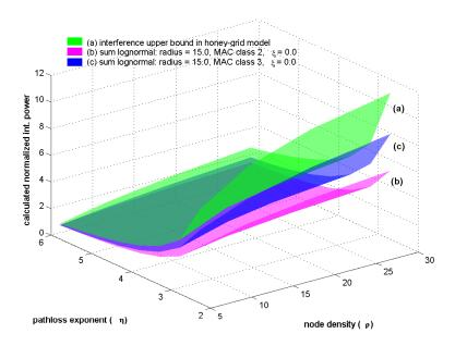
Figure 9.6: Comparison of interference upper bound (9.6) with interference calculated using the lognormal summation method. In this plot we have assumed  $\xi = 0$ .
