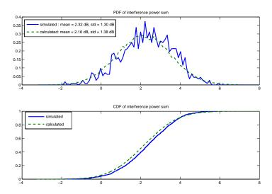
Figure 8.8: Simulated and calculated PDF and CDF of normalized interference power in the center of a circular area with the same parameters as in Figure 8.7.
