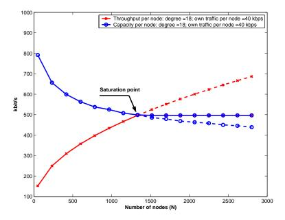
Figure 10.8: Comparing the capacity and the output bit rate per node. In this figure the node's reach, a, is 2 (18 neighbors per node). Other assumptions are the same as in Figure 10.7.
