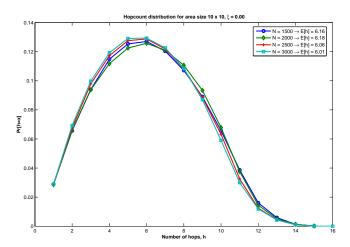
Figure 5.4: Hopcount in an ad-hoc network for  $\xi=0$ , service area is  $10\times 10$  and different number of nodes.
