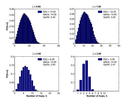
Figure 5.2: Hopcount for different values of  $\xi$ . In all subplots N=1000, and service area is  $20 \times 20$ . The mean hopcount is indicated on each subplot for the ad-hoc network, a lattice of size  $21 \times 21$ , and a random graph with 1000 nodes and the same link probability as in the ad-hoc network.
