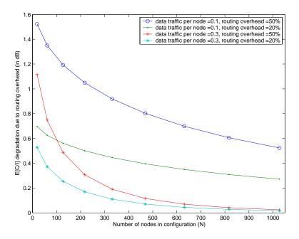
Figure 10.6: Effect of traffic increase due to routing overhead on E[C/I] in an ad-hoc network with different number of nodes. In all cases a=1,  $\eta = 2.4$ , and processing gain is 10.4 dB.
