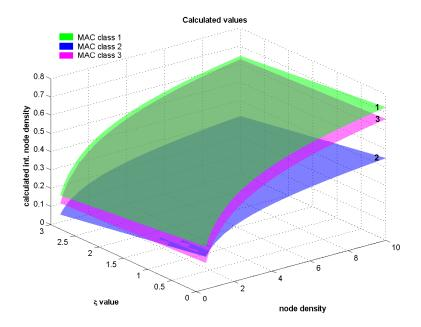
Figure 8.4: Estimated interfering nodes densities using (8.1) for MAC classes 1, 2 and 3.
