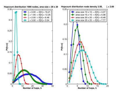
Figure 5.3: Effects of the changes in  $\xi$  (figure on the left) and the area size (figure on the right) on the hopcount in ad-hoc networks.
