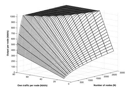
Figure 10.9: Throughput per node for different values of input data bit rate per node and different number of nodes. Each node's own traffic varies between 10 kbps and 80 kbps. Other values and assumptions are the same as in Figure 10.7.
