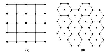
Figure 9.2: Regular lattice forms in the 2-dimensional plane: (a) rectangular lattice, (b) hexagonal lattice.
