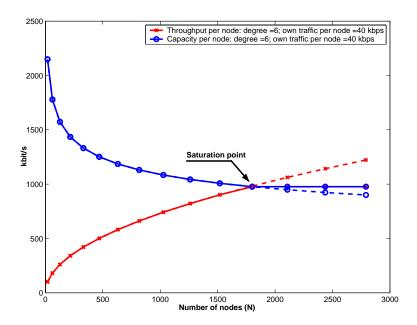
Figure 10.7: Comparing the capacity and the output bit rate per node. In this figure the node's reach, a, is 1 (6 neighbors per node) and each node's own traffic equals to 40 kbps. For calculations we have assumed: channel bandwidth B is 22 MHz (before despreading), processing gain g is 11, data packets size P is 1000 bytes, transmission speed r is 2 Mbps,  $t_0 = 364\mu s$  and the pathloss exponent  $\eta$  is 2.4.
