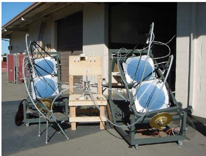
Figure 2.5: The experimental test set up with fibre optical cables [23]
