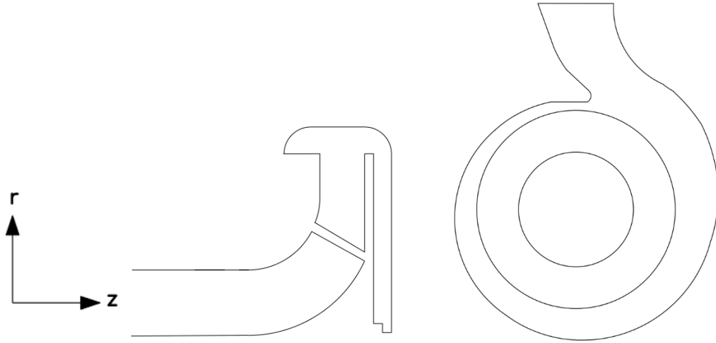
Figure 3.4: Sketches of the volute used in the simulations. On the left meridional plane view, to underline the absence of the leakage flow, on the right the complete volute as seen from the -z axis direction.
