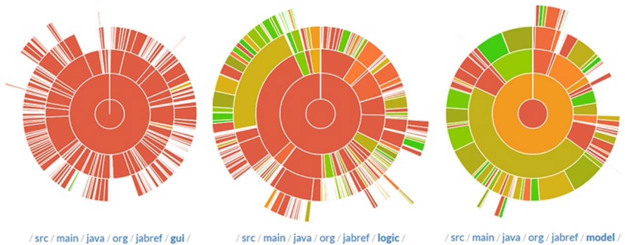
Figure 3: Sunbursts of the GUI, Logic, and Model package. Red indicates code covered for less than 70%, whereas code covered between 70% and 100% is a gradient from orange to green.
