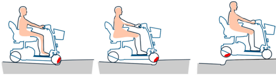
Fig. 5. A risky moment after having entered the road: being unable to re-mount the higher curb on the other side and getting stuck on the road, exposed to oncoming traffic. After this happened to MOSa, he took a run-up and mounted the curb forcibly. This first compresses the front of the body, then presses the body into the seat, and then launches the body out of the seat and the mobility scooter's back wheels into the air. See also Appendix B1 .
