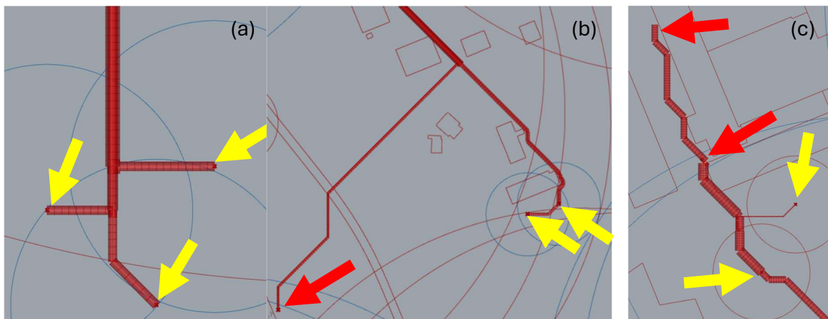
Figure 6: (a) pipe sizing growing after each well, (b) impact of pipe sizing because of supply and demand, (c) solved pipe sizing problem
