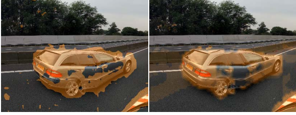
Figure 3: Results from features extracted from FC-VGGNet (first) and VGGNet (second). Features from FC-VGGNet are well-localized and have strong activations.
