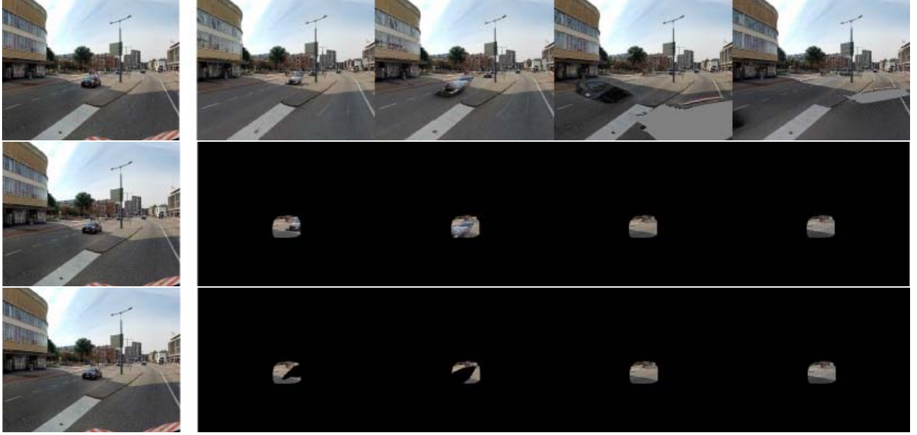
Figure 4: Images in the first column are the input images ( I_t ) at time t . The first row contains images \hat{I}_{t' \rightarrow t}^r for t' \in \{-2, -1, +1, +2\} that is projected to the view point of I_t . Results in the second row are obtained after removal of regions around the area of interest. Finally, the third row ( \hat{I}_{t' \rightarrow t}^r ) is obtained after removal of moving objects from other views.
