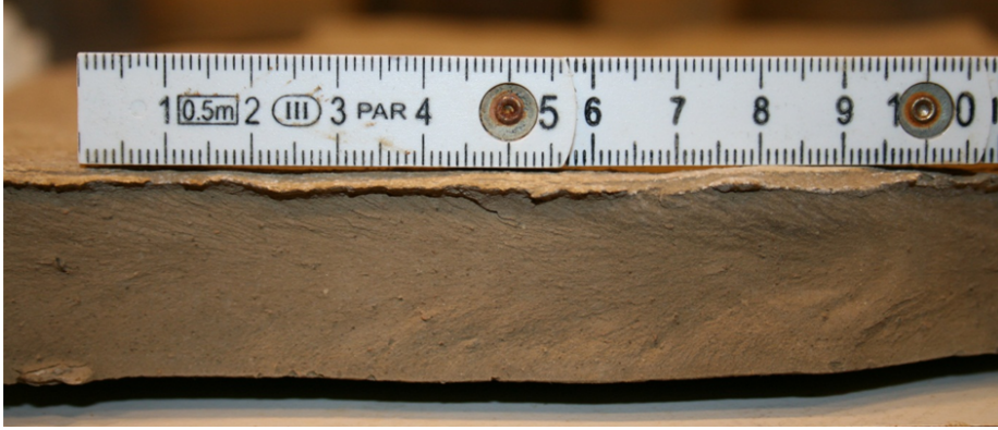
Figure 2.10: Plumose structures in fractures from container with a 50 mm initial clay thickness.
