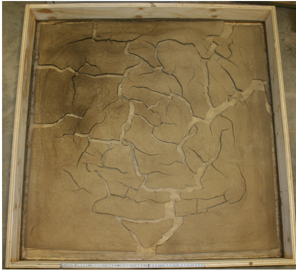
Figure B.7: Crack pattern in 1 x 1 m board with 20 mm initial thickness and an initial water content of three times liquid limit approx. (170%).
