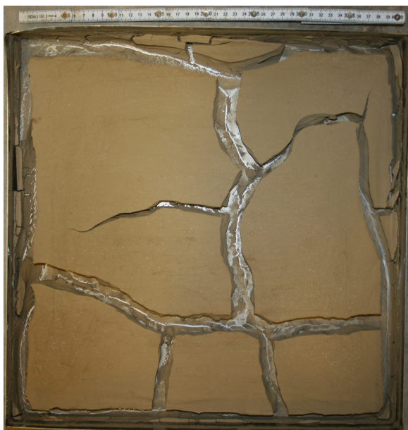
Figure B.10: Crack pattern in 0.4 x 0.4 m board with 40 mm initial thickness and an initial water content of twice the liquid limit approx. (114%).
