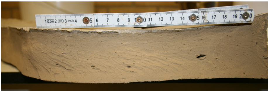
Figure 2.11: Plumose structures in fractures from container with a 100 mm initial clay thickness.
