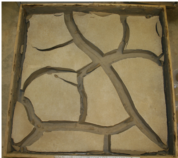
Figure B.9: Crack pattern in 1 x 1 m board with 100 mm initial thickness and an initial water content of twice the liquid limit approx. (114%).
