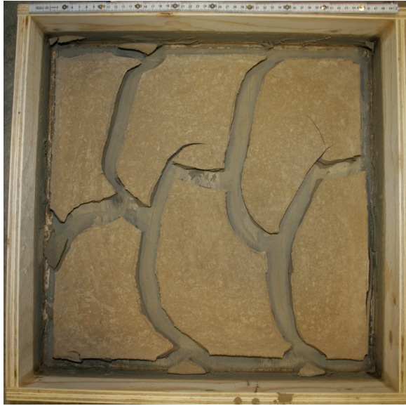
Figure B.5: Crack pattern in 0.5 x 0.5 m board with 50 mm initial thickness and an initial water content of three times liquid limit approx. (170%).
