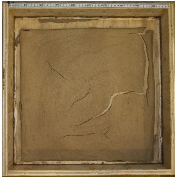
Figure B.4: Crack pattern in 0.5 x 0.5 m board with 20 mm initial thickness and an initial water content of three times liquid limit approx. (170%).
