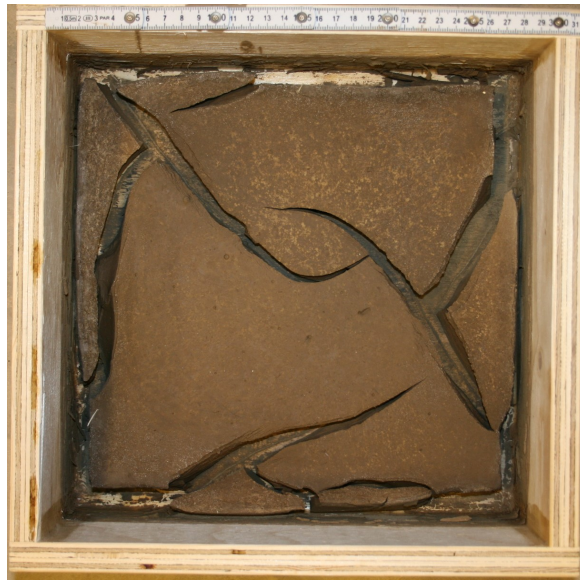
Figure 2.3: Cracking in 0.3 x 0.3 m board with 50 mm initial thickness and an initial water content of three times liquid limit approx. (170%).
