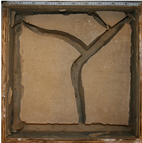
Figure B.6: Crack pattern in 0.5 x 0.5 m board with 100 mm initial thickness and an initial water content of twice the liquid limit approx. (114%).
