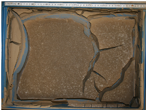
Figure B.13: Crack pattern in 0.35 x 0.5 m board with 50 mm initial thickness and an initial water content of three times liquid limit approx. (170%).
