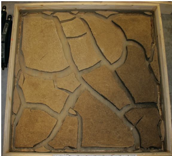
Figure B.8: Crack pattern in 1 x 1 m board with 50 mm initial thickness and an initial water content of three times liquid limit approx. (170%).
