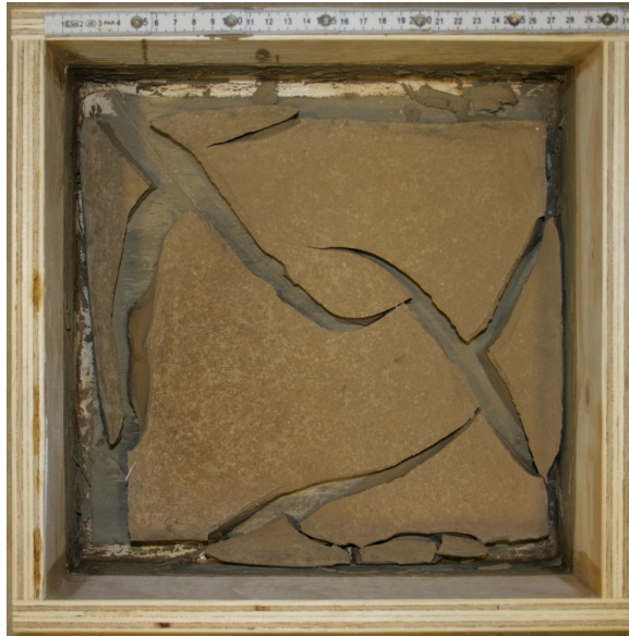
Figure B.3: Crack pattern in 0.3 x 0.3 m board with 50 mm initial thickness and an initial water content of three times liquid limit approx. (170%).
