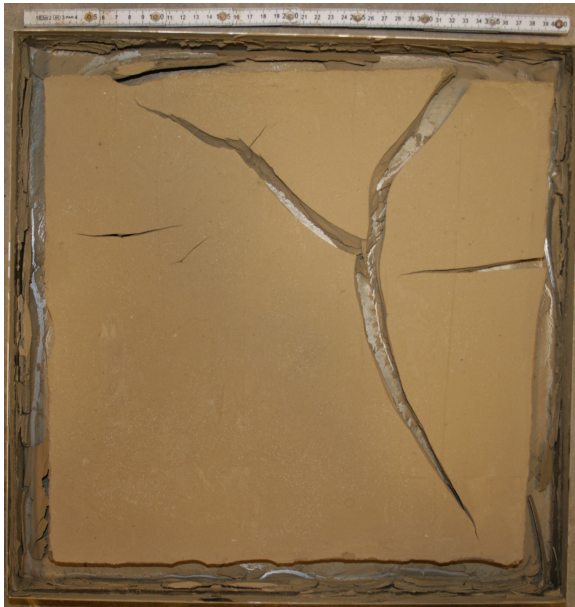
Figure B.11: Crack pattern in 0.4 x 0.4 m board with 40 mm initial thickness and an initial water content of three times liquid limit approx. (170%).
