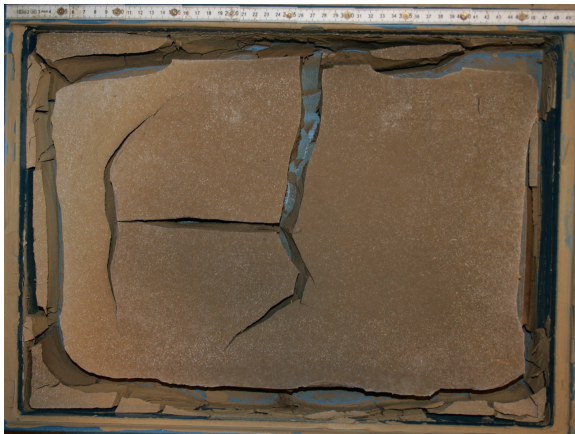
Figure B.12: Crack pattern in 0.35 x 0.5 m board with 50 mm initial thickness and an initial water content of twice the liquid limit approx. (114%).
