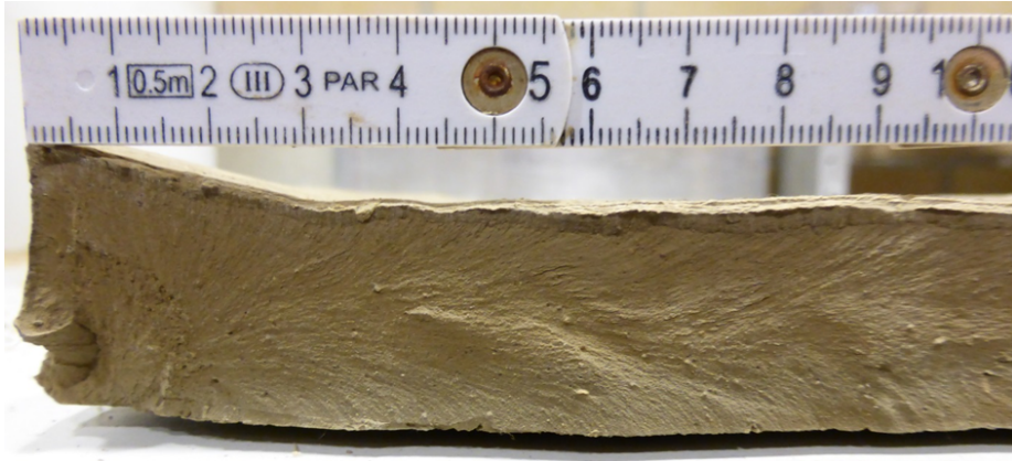
Figure 2.13: Example of a fracture starting at the bottom left corner of the layer and advancing under the surface towards the right.
