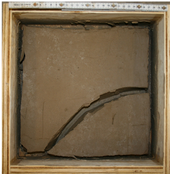
Figure B.2: Crack pattern in 0.3 x 0.3 m board with 50 mm initial thickness and an initial water content of twice the liquid limit approx. (114%).
