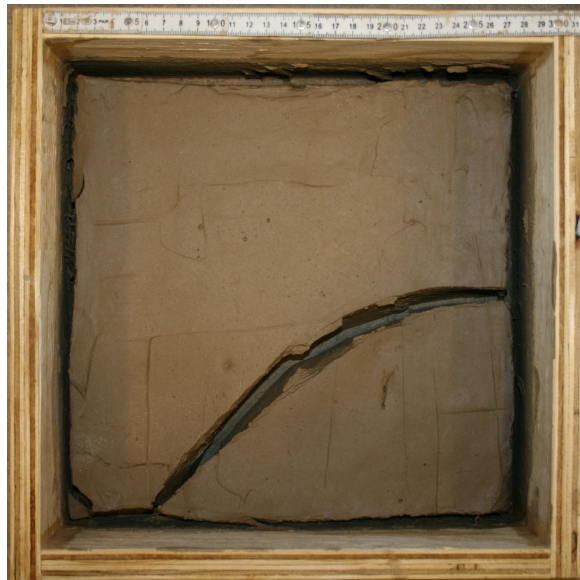
Figure 2.4: Cracking in 0.3 x 0.3 m board with 50 mm initial thickness and an initial water content of twice the liquid limit approx. (114%).
