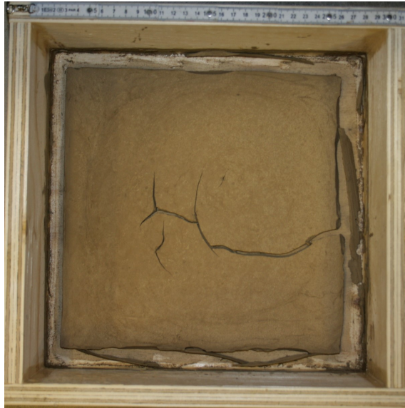
Figure B.1: Crack pattern in 0.3 x 0.3 m board with 20 mm initial thickness and an initial water content of three times liquid limit approx. (170%).
