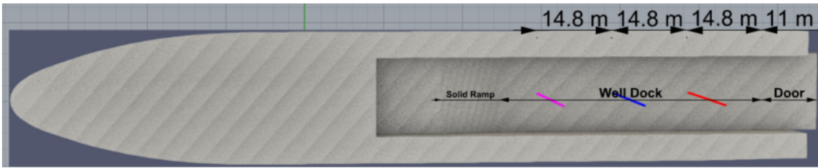
Figure 7.8: Wave probes located within the well dock for the results exportation and their coordinates are found in table 7.5
