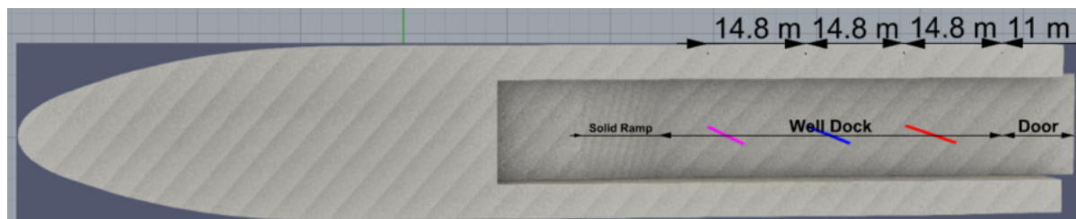
Figure 4.4: Model test set-up LPD-Wave Probes 1-3
