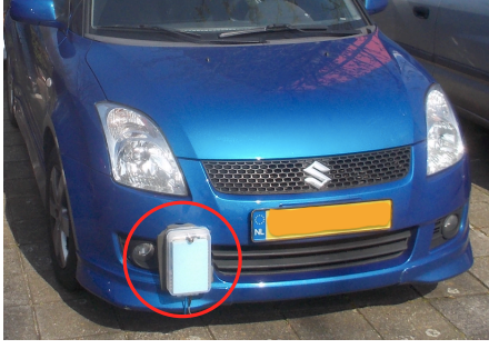
Fig. 2: Experimental auto equipped with NXP radar demonstrator
