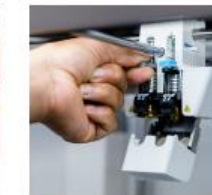
Print core CC Ruby-tipped for printing abrasive composites
