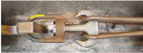
Figure 79: 3D printed hook during its load test, Huisman
