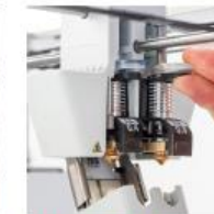
Print cores AA and BB Quick-swap nozzles for build and water-soluble support materials
