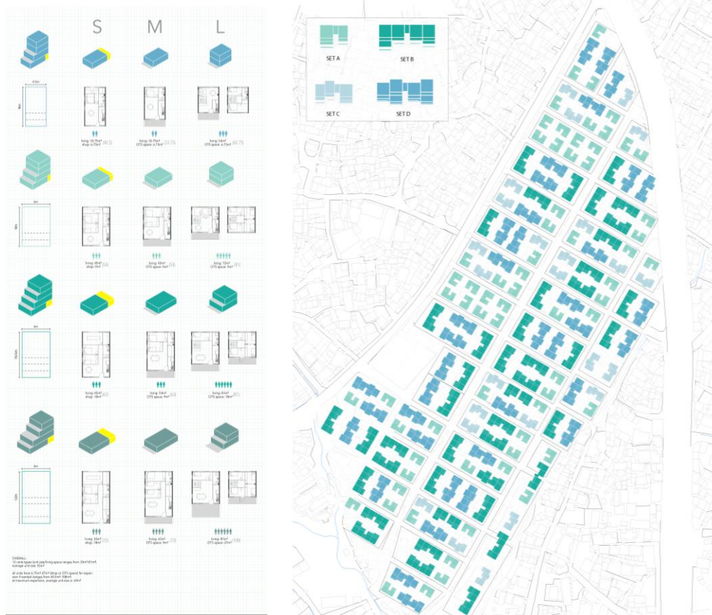
Figure 4 – A huge variation of combinations in the urban scale (right) created by four sets composed by four different unit blocks (left)
