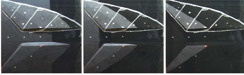
Figure 5.1 – Water rising up on the reef. From left to right: water depth is 10, 20 and 30cm.
