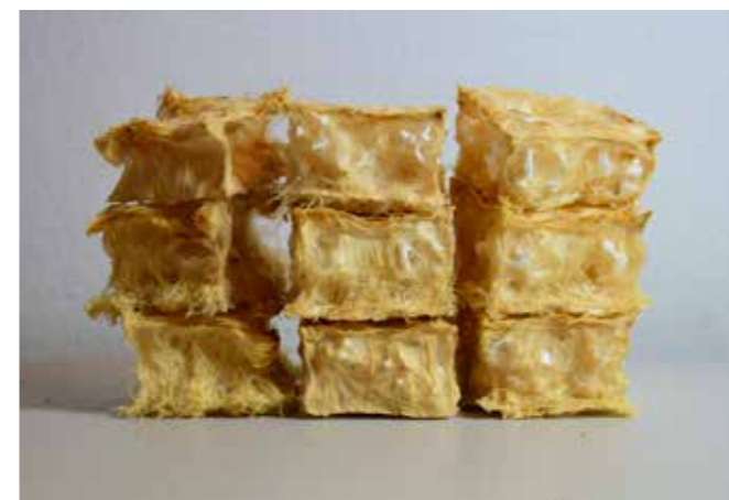
Figure [90]. Compression test samples, from left to right: naturally grown, with 10 pieces of 14mm beads, with 6 pieces of 20mm beads
