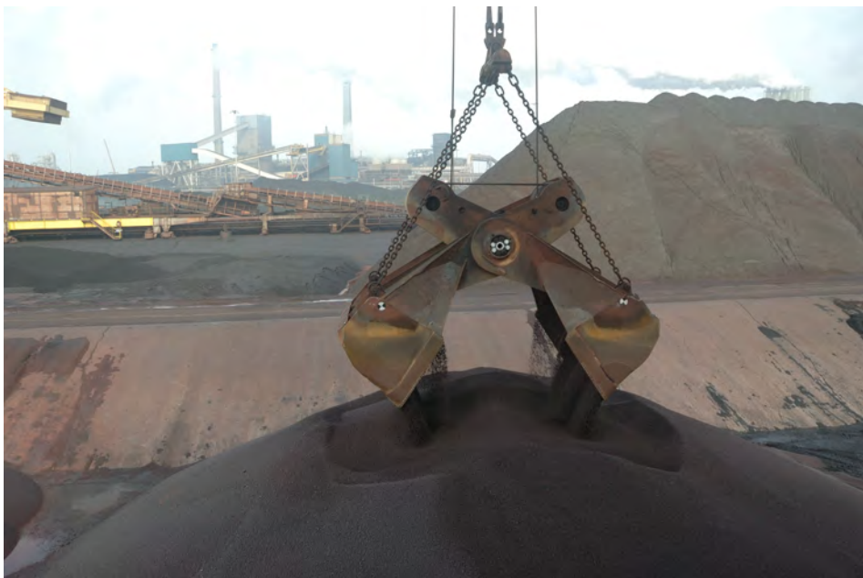
Figure 2.9: A Nemag Scissors grab releasing iron ore.
