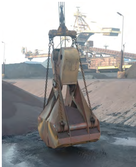
Figure 3.5: Angle of repose on top of a grab.
