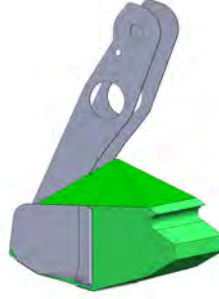
Figure 8.3: Definition of maximum capacity of grab V_{\text{grab}} .
