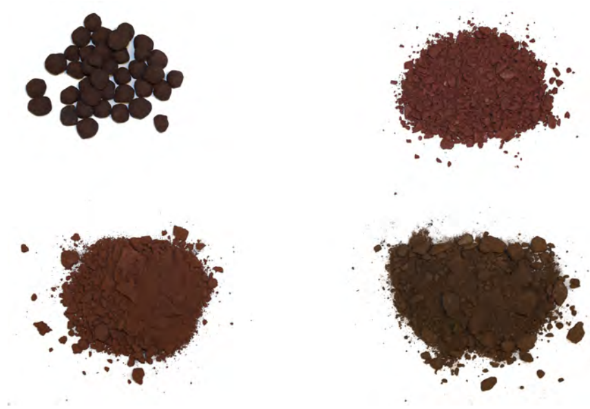
Figure 3.1: Test materials. Clockwise, starting top left: iron ore pellets, Sishen , Carajas and SSFG.
