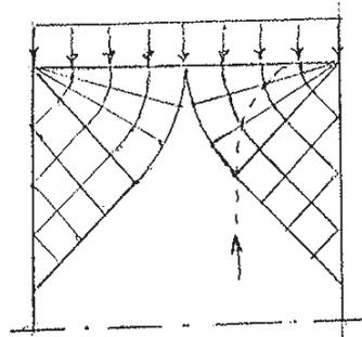
For long blocks with respect to the bearing plates the maximal spreading will occur at both plates according to the figures below.
