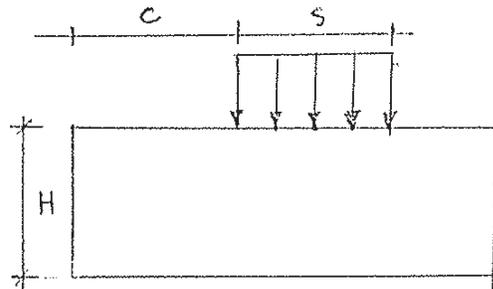
When  $c/H = (L - s)/2H \geq 1.5$ , thus when  $L \geq 3H + s$ , the maximal spreading is reached according to the table and to the first figure above of [1]. (This indicates friction
