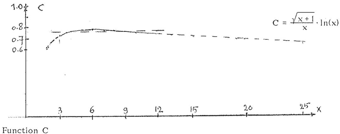
and because  $\sigma_s \cdot s = \sigma_0 \cdot L$  (see figure below) is:  $\sigma_s(1 - s/L) = 2.48 \cdot k \cdot \ln(2H/s)$ . Further the construction for a finite block gives the indication that the spreading of the stress is below:  $L \approx 2H + s$  or:  $H \approx (L - s)/2$  when  $H > s$ , thus:  $L/s > 3$  (Below this value the spreading is less strong and finally failure is similar to the cube test). Substitution of the values for  $\sigma_0$  and  $H$  in eq.(4) gives:
