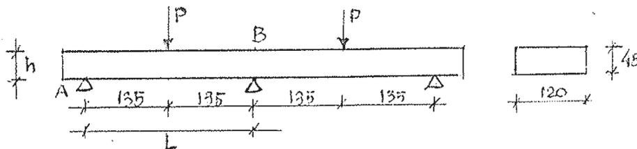
For the beam on 3 supports a cut of the beam at the middle support at point B will give a rotation at B by the loading P of:  $\varphi = PL/16EI$ . The shear strain will give no rotation at B. Because the beam is fixed at point B the moment at the support will
