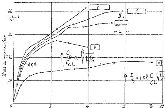
Bearing strength  $\perp$ , specimen 15x15 cm, lengths: 15, 30, 45, 60, 75 cm, of a to e, [1]
