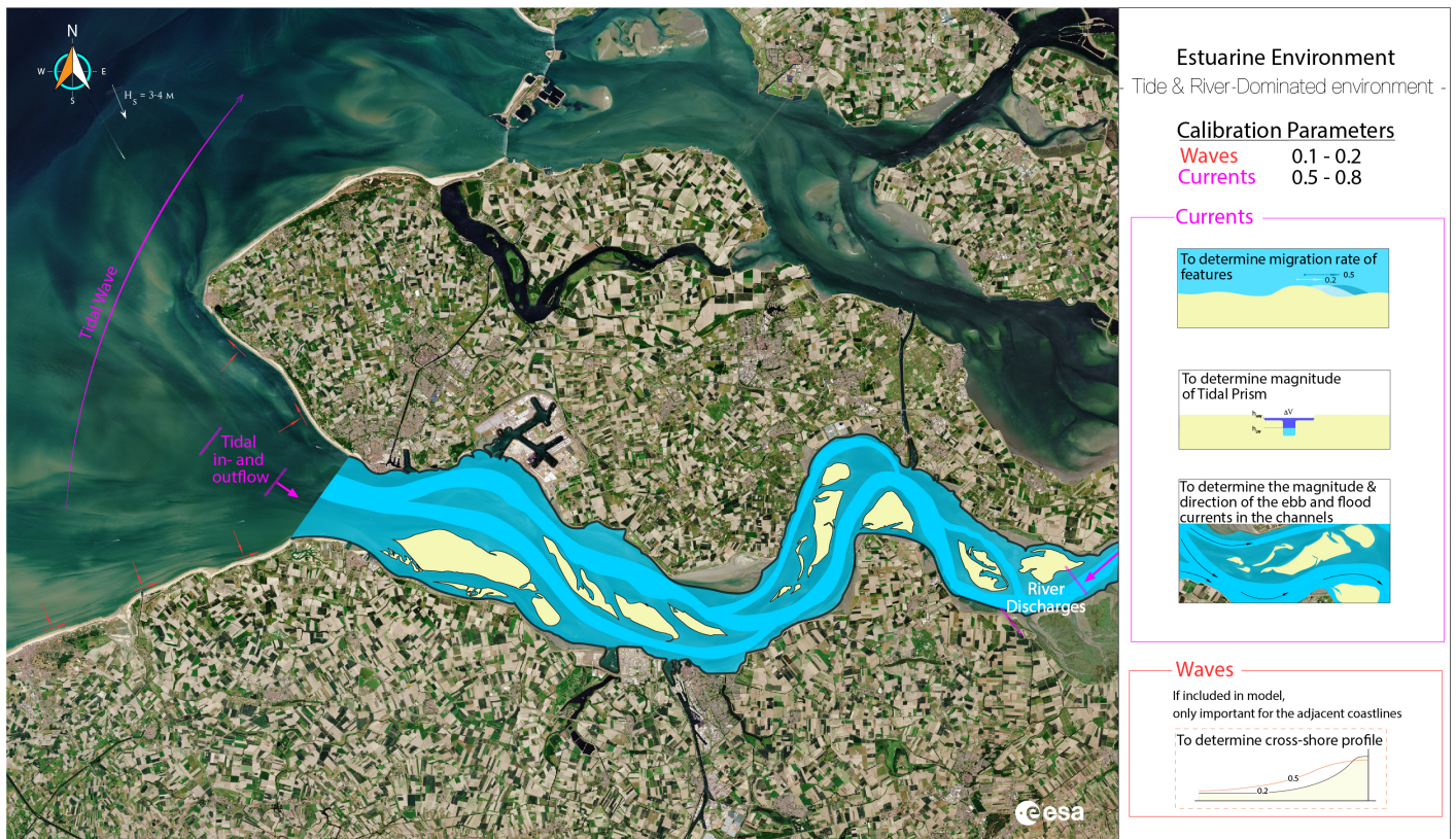
Figure 39: A schematic overview of the Western Scheldt Estuary, illustrating hereby the important physical processes and the associated modelling strategy.
