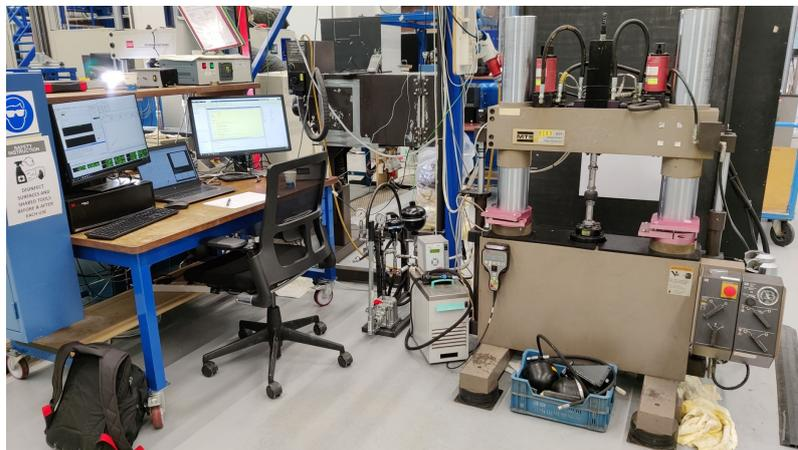
Figure 10.1: MTS Elastomer Test System 831
