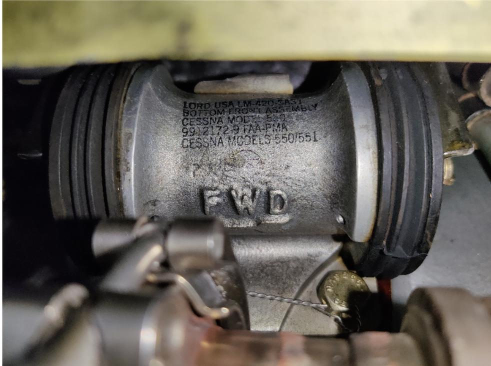
Figure 5.2: Lower engine mount of PH-LAB engine 2
