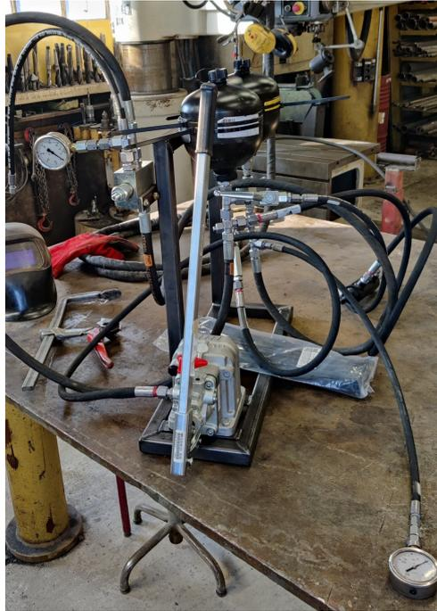
Figure 10.6: Hydraulic components stand construction
