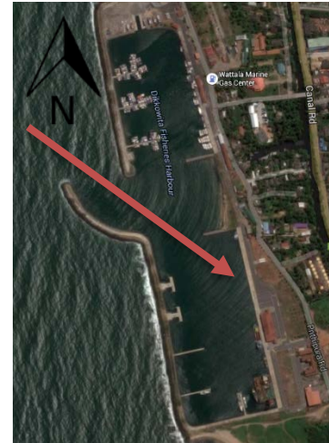
Figure 57 Flow direction of the water into the southern basin (Google, 2015)
