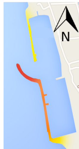
Figure 20 Overview of the dangerous parts of the breakwater for the yachts and pedestrians with respect to overtopping (Google, 2015)
