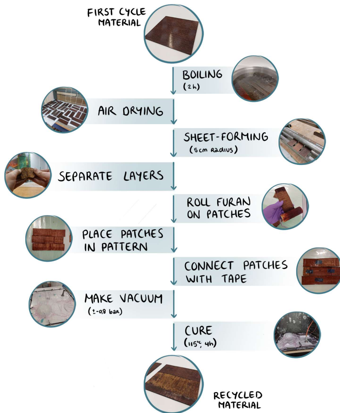
Figure 13: Making process diagram of recycled material
