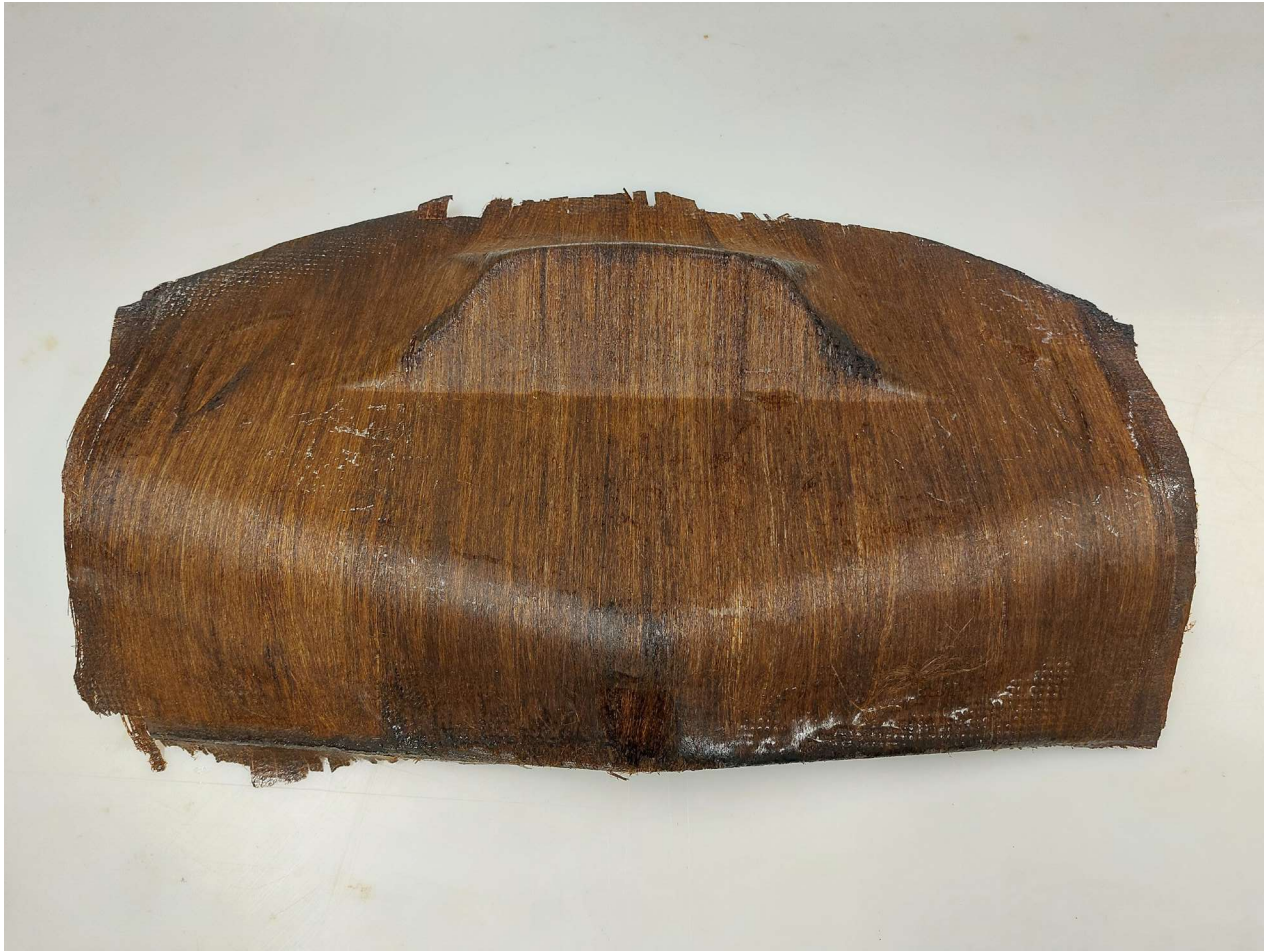
Dashboard produced with first-cycle material.
