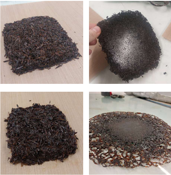
The sample on the first row has a fibre content of 50%. The sample on the second row has a fibre content of 35%.
