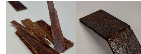
Figure 15: Sheet-forming first-cycle (left) and recycled (right).
