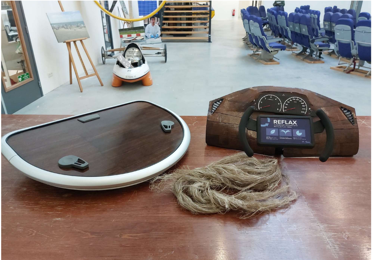
Deck hatch made of first-cycle flax/furan, next to a bundle of flax and the dashboard produced with recycled flax/furan.
