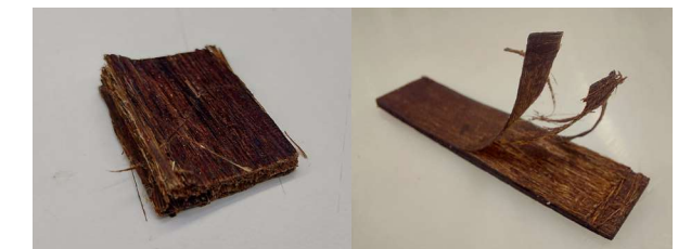
Figure 18: Boiling first-cycle (left) and recycled (right) material.
