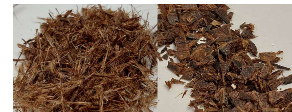
Figure 17: Granulating first-cycle (left) and recycled (right).
