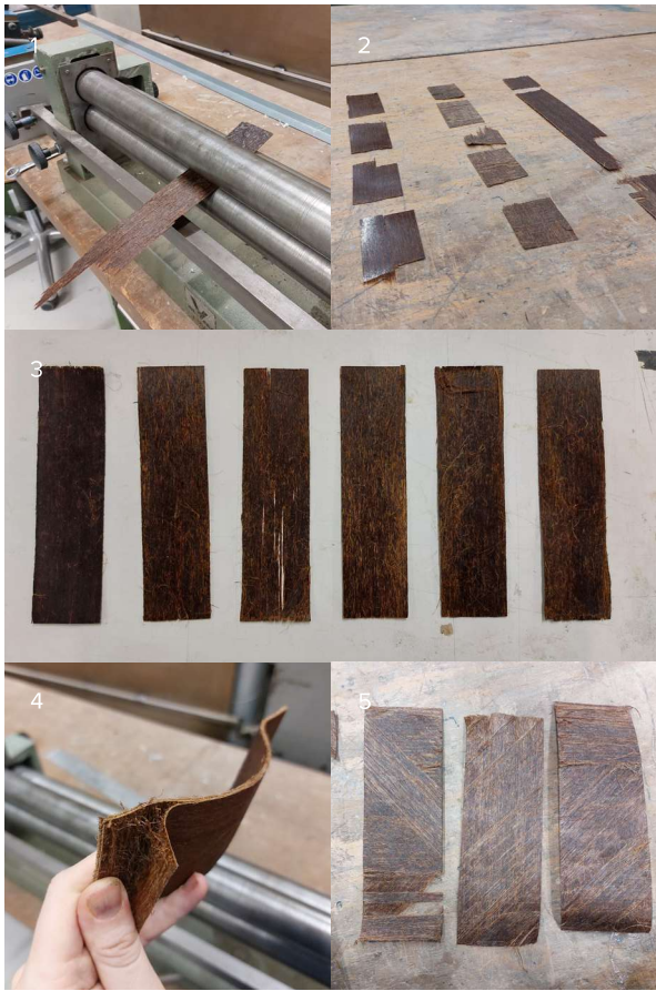
Figure 10: Separating layers by putting material through sheet-forming machine (1). Separating without boiling (2), after boiling (3), with a curved lay-up (4), and a with multi-directional lay-up (5)
