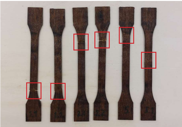
Recycled specimen with break lines
