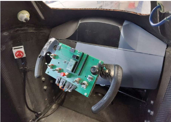
Figure 43: 3D printed version of dashboard
