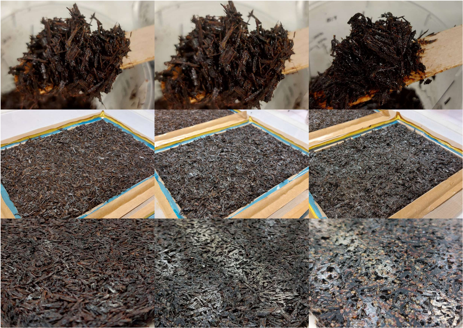
Figure X: First row shows a granulate mixed with furan resin, second row shows the mould prepared with teflon sheet, third row shows the produced sampels after curing in the oven. For each row, from left to right, 50%, 35%, and 20% fibre content.
