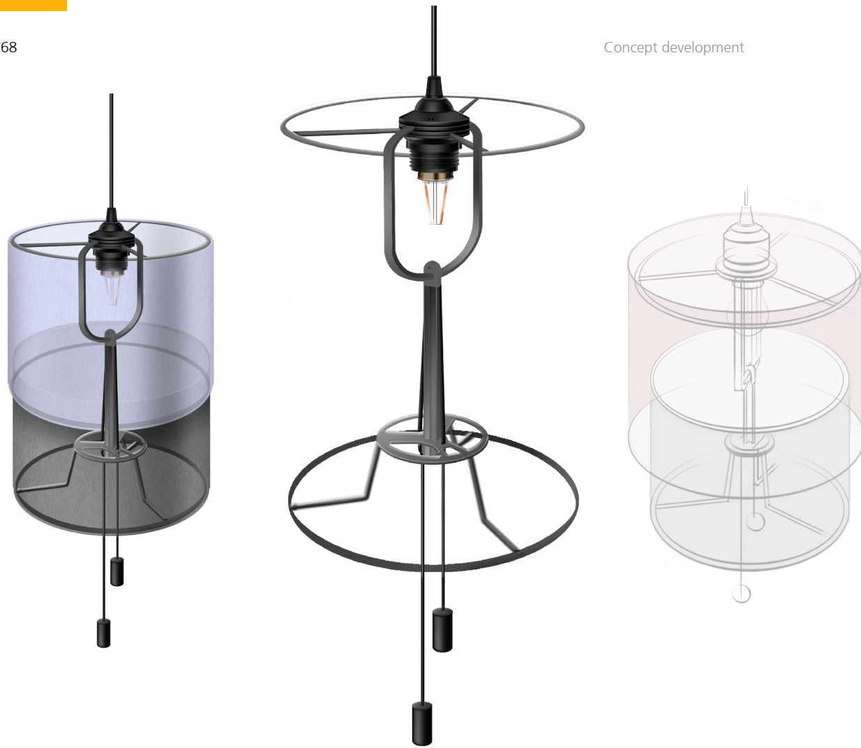
Figure 3.16 Sketches of the insides of the lampshade based on IKEA pendant
