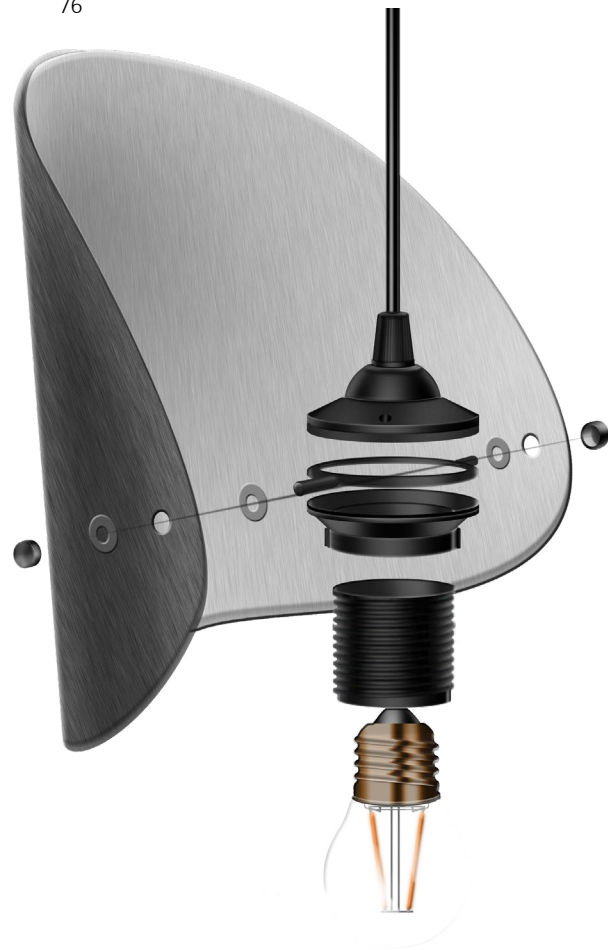
Figure 3.23 Exploded view depiction of the Petal light design.
