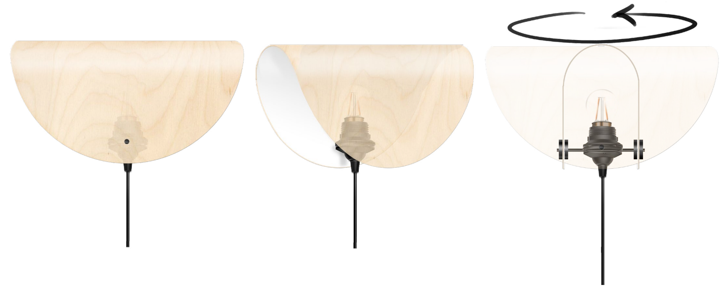
Figure 4.43 Illustration shows the rotation without the hinge feature.
