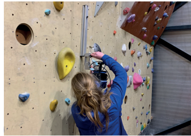
Attach the Meta-Grip to the rail.
