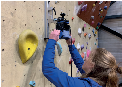
Turn the Meta-Grip in the correct angle for the measurement.
