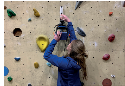
Adjust the Meta-Grip to the correct height.
