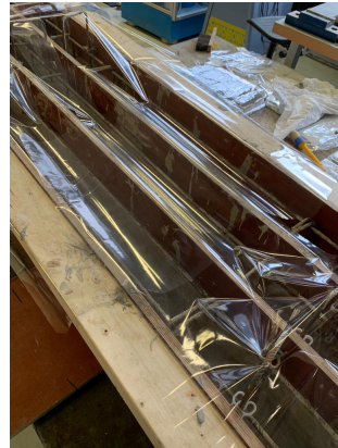
Figure 3.19: Covering to retain moisture
