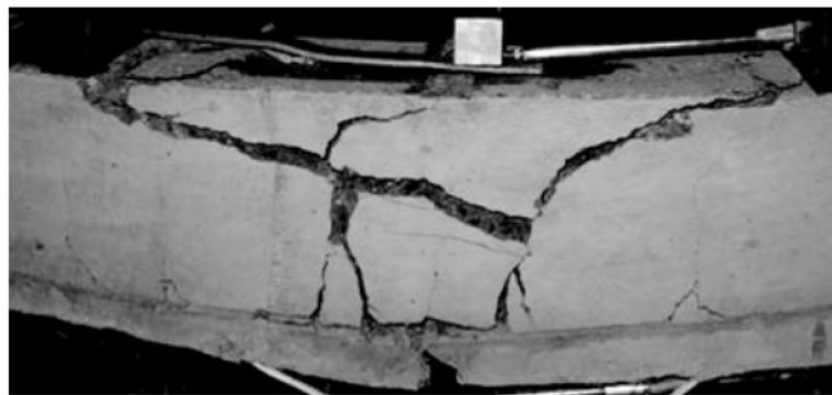
Figure 2.11: Crack opening in UHTCC25 specimen [7]
