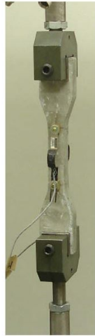
Figure 2.20: Uniaxial test set-up [10]
