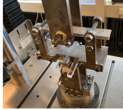
(b) Four-point bending test before loading
