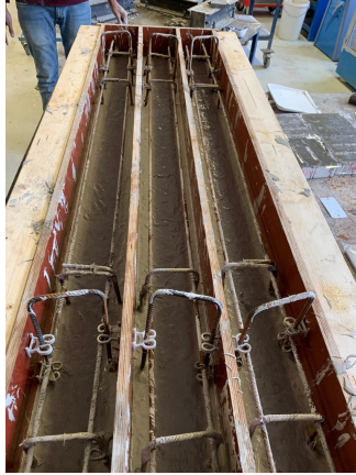
(a) Casting of SHCC layer
