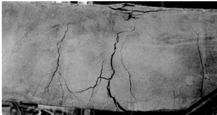
Figure 2.14: Crack opening in UHTCC15 specimen [7]
