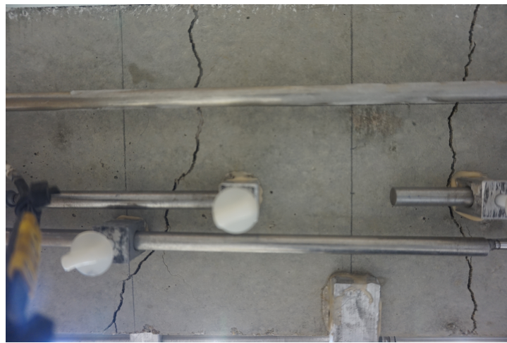
Figure 3.35: Image of cracks on the bottom-side of CC beam (Load step 60 kN)
