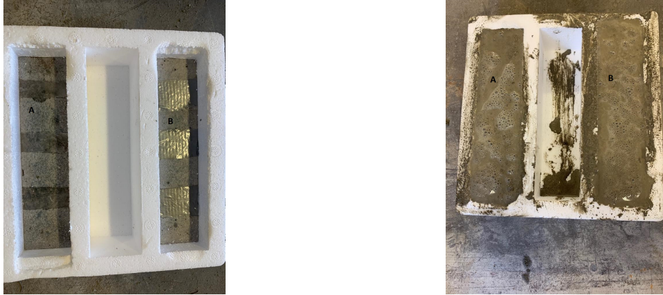
(a) Application of Vaseline strips (left) and tape (right) (b) Pouring normal concrete layer on both specimens
