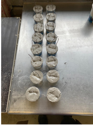
(a) Casting of SHCC spacers
