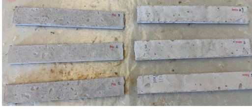
(a) Specimens of SHCC with PVA (Left) and HMPE (Right) fibers
