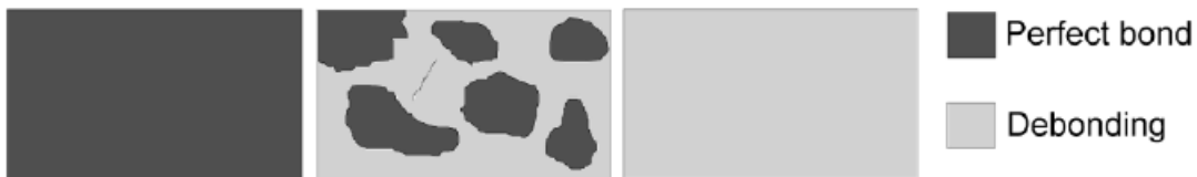
Figure 2.6: Types of bonding at the interface [4]
