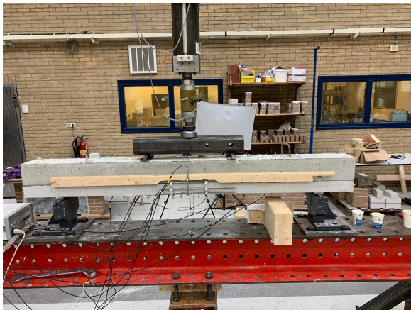
(a) LVDT arrangement to measure deformation
