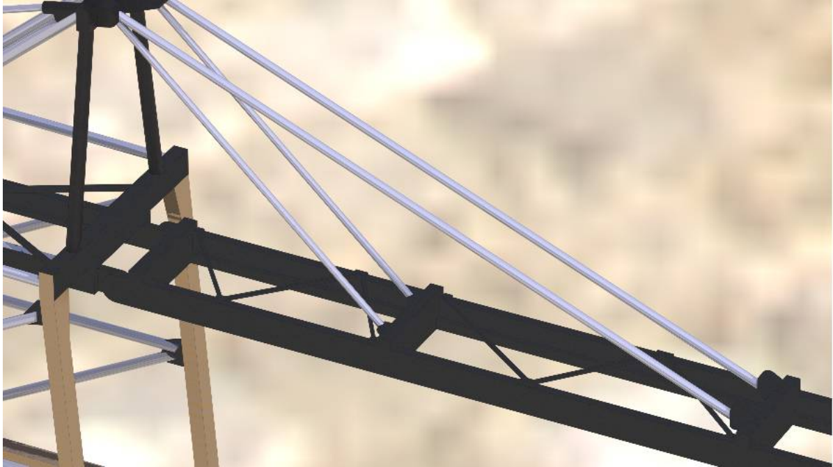
(a) Detail of the forestay digital model. Note how the hinges are taken out of the forestay in the digital model and the forestay is modelled as perfect rods.
