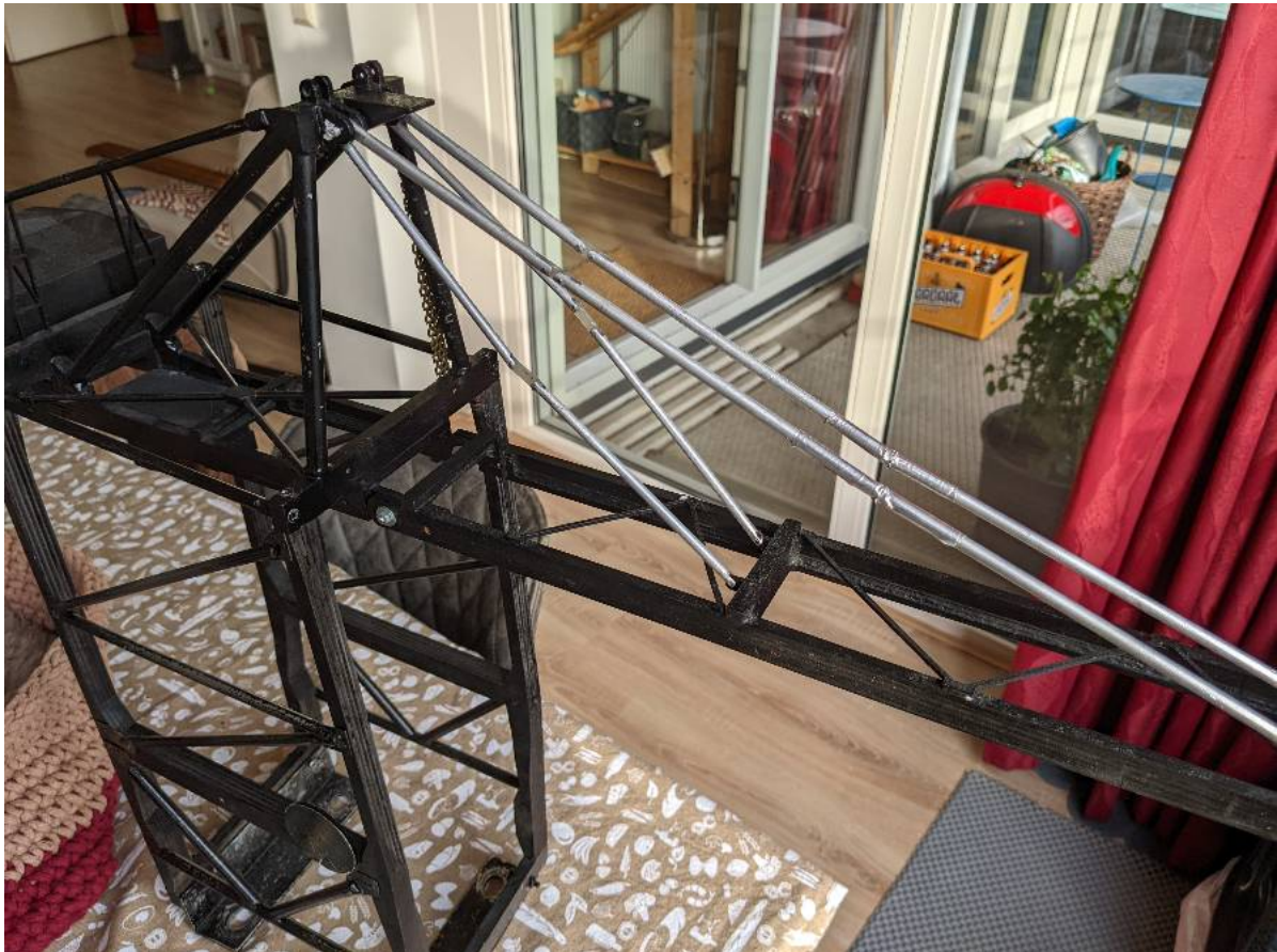
(b) Detail of the forestay wind tunnel model
