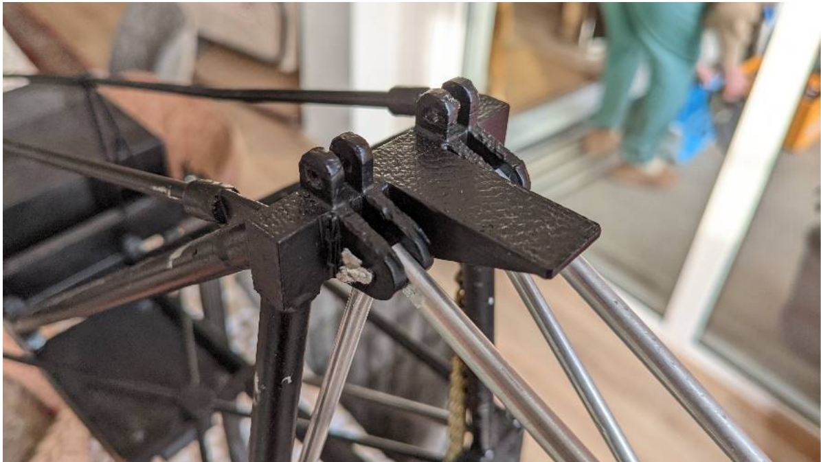
(b) Detail of the apex beam wind tunnel model
