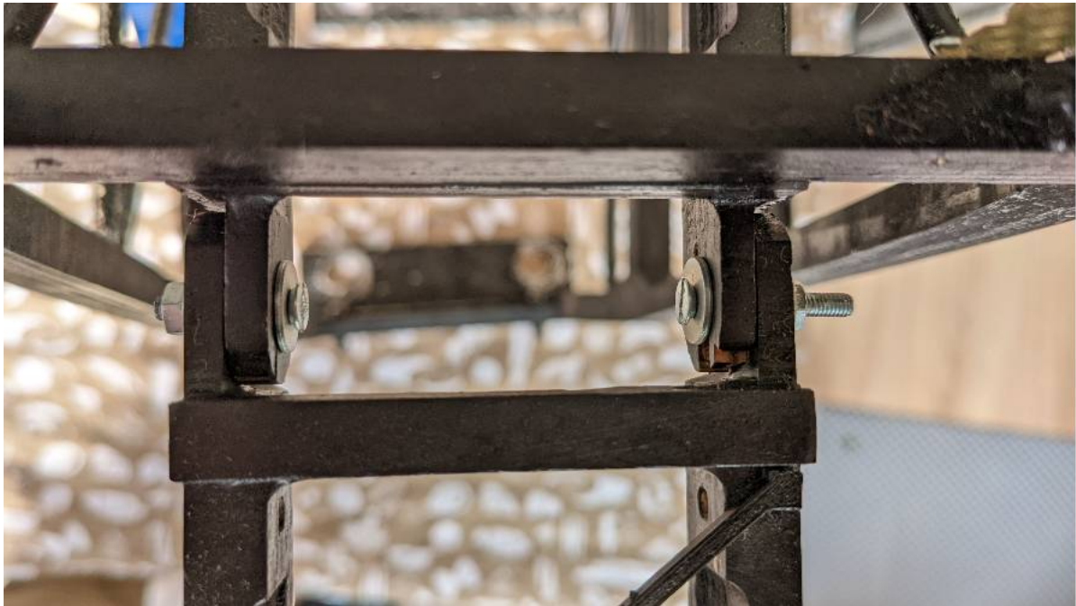
(b) Detail of the boom hinge wind tunnel model
