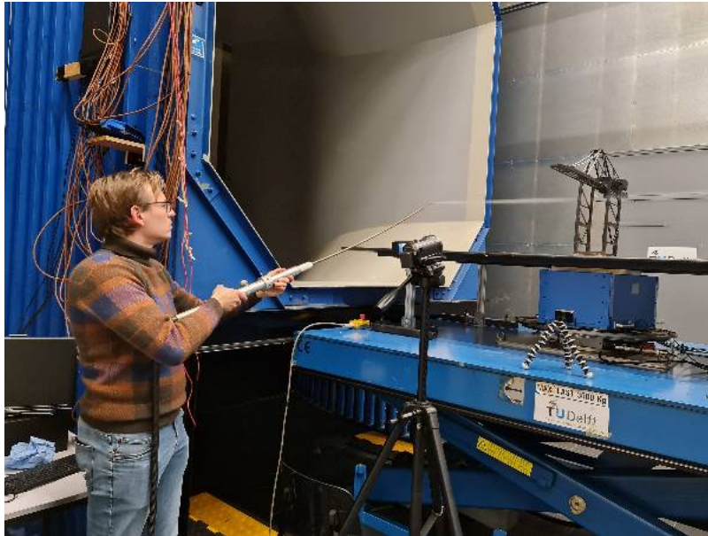
(a) Testing with the smoke generator, several cameras used for capturing the smoke trail are also visible in this photo.
