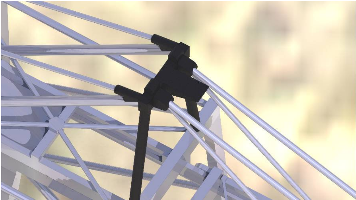
(a) Detail of the apex beam digital model. Note the simplified geometry compared to the wind tunnel model.
