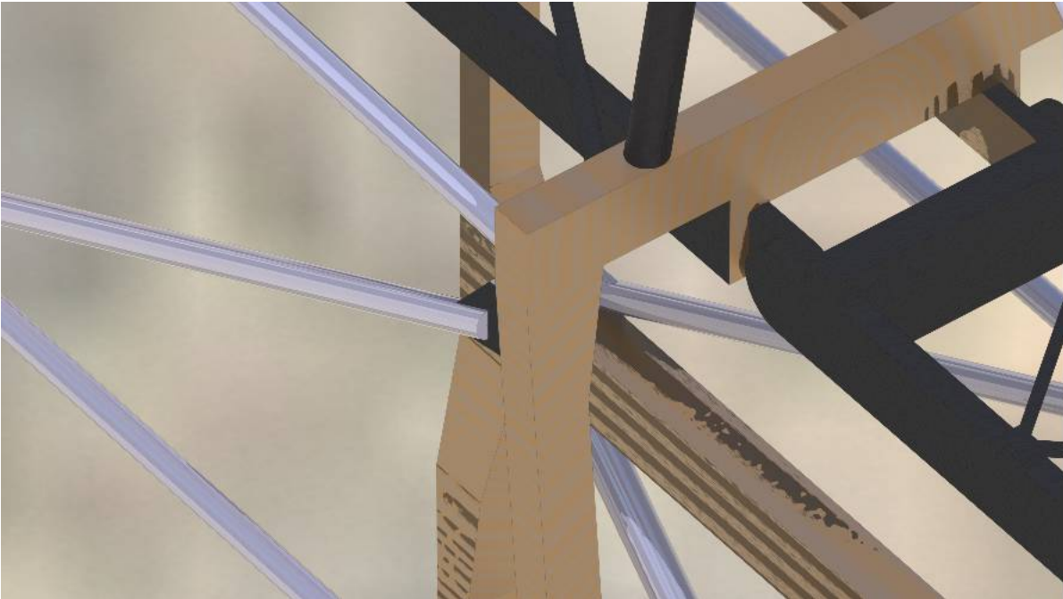
(a) Detail of the portal beam digital model. Note how the geometry is absent of screws and gaps, present in the wind tunnel model.
