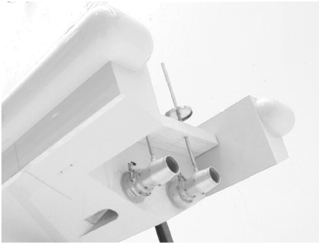
Fig. 13. View of the waterjets arrangement on the NH-1816 model.
