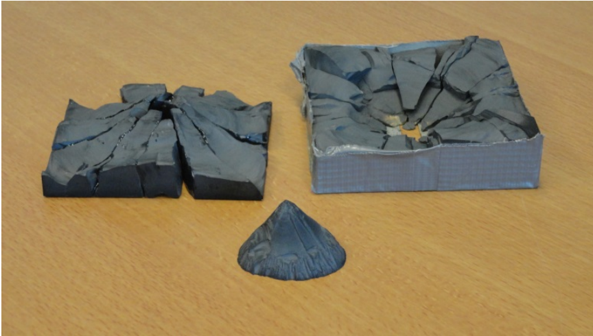
Figure 1.3: Silicon carbide ceramic tile, subjected to a single projectile impact. Cone cracking and radial cracking in the ceramic target is clearly visible. (E. Carton, TNO Laboratory for Ballistic Research, personal communication)
