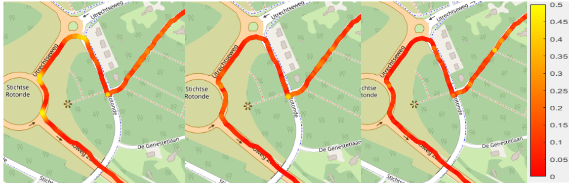
Figure 7. Snapshots of heat maps of lateral (left), longitudinal (middle), and gravitational acceleration (right). The scale ranges from 0 g (red) to 0.5 g (yellow).
