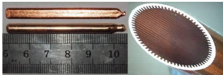
FIGURE A.3: The micro-grooved heat pipe and its grooves [166].
