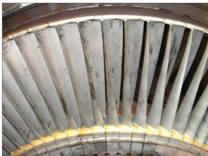
Figure 2.11: Twisted blades in the third turbine stage
