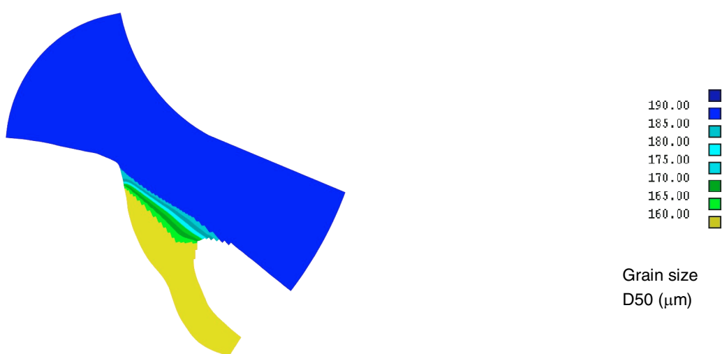
Figure 4.1 Grain size 190 \mu\text{m} (Ganges) to 160 \mu\text{m} (Gorai) applied in model grid
