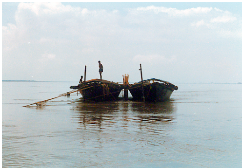
Figure 5 Floating-screen test by Jamuna Test Works Consultants using vertical screens mounted between country boats
