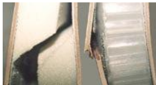
Figure 58: Foam core (left) and honeycomb (right). Retrieved from Carbon-core (Carbon-Core Corporation, 2020)
