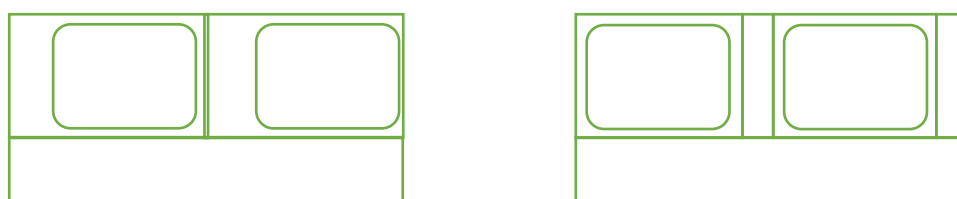
Figure 59: Panel configurations that combine SGMm and ICMm/ICRm layout (left) and minimize window frame area (right)
