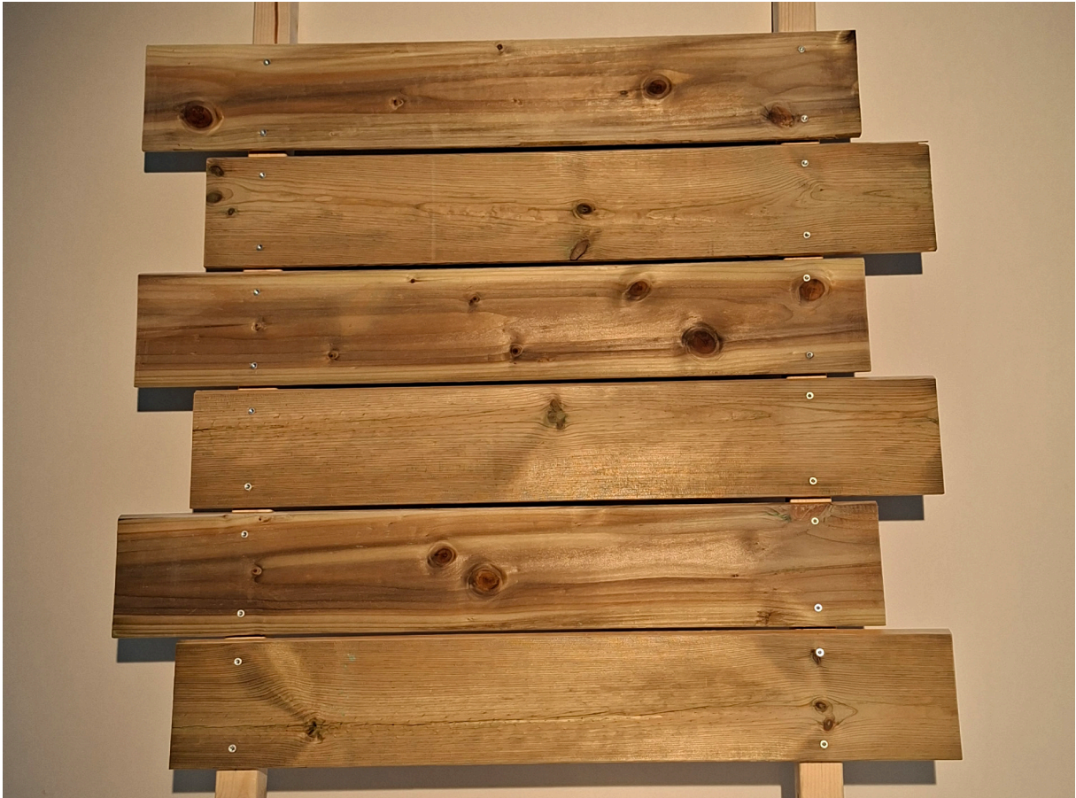
FIG 77. Physical model open joint horizontal cladding (1:1 scale)
