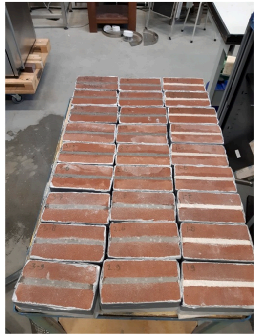
Fig. 1. Example of sealed and pointed test specimens.
