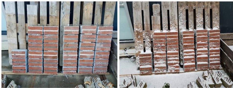
Fig. 4. Test specimens in outdoors exposition. Left October 11, 2018, right January 21, 2019.
