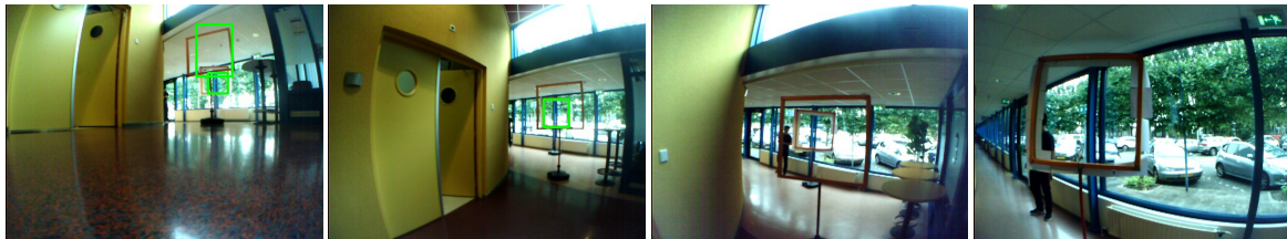
Figure 4.13: Predictions in the Hallway environment of the network trained with distortion. In some images (1 and 2) the network predicts a half way correct bounding box. Yet in the majority of images such as 3 and 4 the gate is not detected, although clearly visible.
