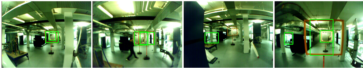
Figure 4.12: Predictions in the Basement environment of the network trained with distortion. The network produces very nice detections in cases of heavy occlusion (1 and 2). However, in other cases where the gate is visible at least equally well (3 and 4) the gate is not detected or with bad localization.
