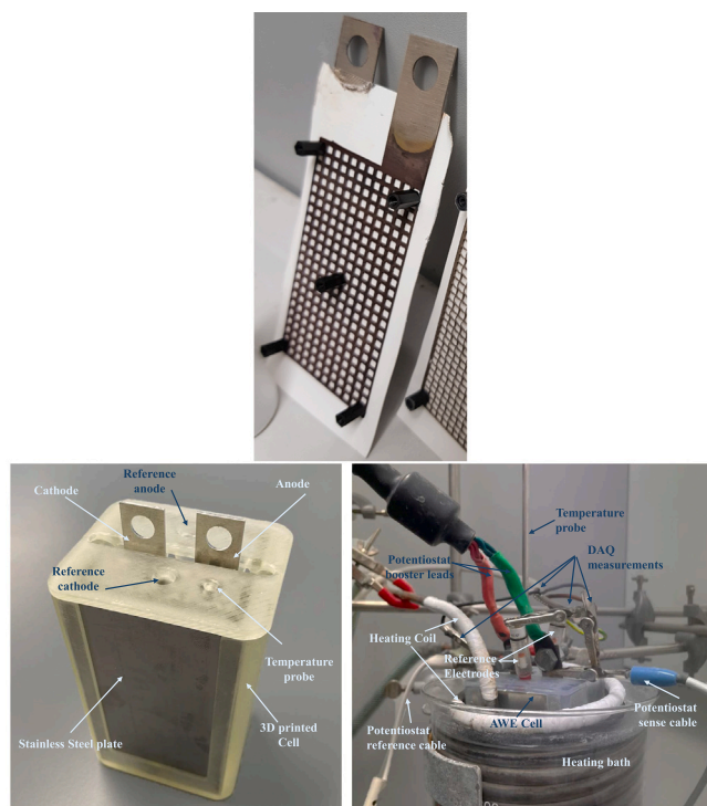
Fig. 1. Top: The L-shaped electrodes were compressed with five nylon bolts onto the diaphragm to approach a zero-gap configuration. Bottom left: The 3D-printed beaker cell with stainless steel end plates, electrodes, and holes for the reference electrodes and temperature probe. Bottom right: The cell was submerged in a heating bath with a coil that can both heat and cool. The booster cables were bolted onto the anode and cathode, and various cables for voltage measurement are shown. The blueish taint on the right, compared to the more yellow colour on the left picture, comes with heating and wetting.
