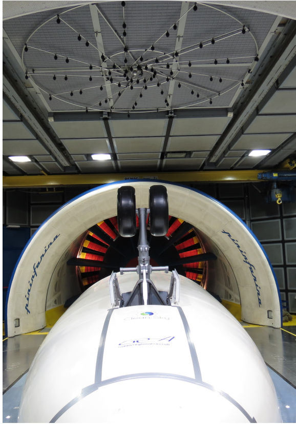
Figure 5.3: ALLEGRA NLG model inside the wind tunnel with the top array visible [17].
