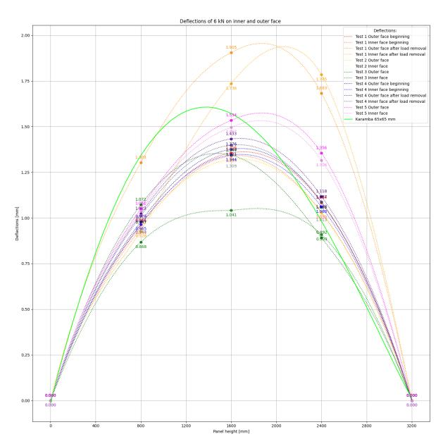
Figure F.1: 6 kN on inner and outer face deflections
