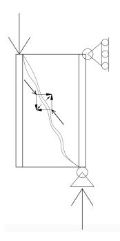
Figure 4.36: Loading case 6 kN on the outer face crack formation/failure
