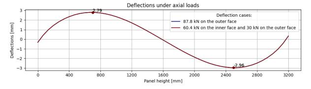
Figure 4.21: Deflections of axial load 87.8 kN and 90.4 kN.
