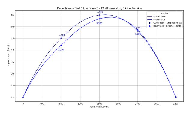
Figure 4.11: Deflections of Test 1 inner face loaded with 12 kN and outer face loaded with 6 kN.
