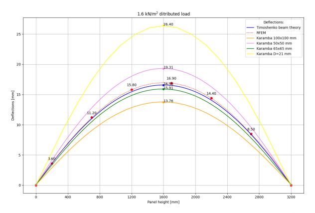
**Figure 4.17:** Karamba3D model scaling with RFEM and Timoshenko beam equations under 1.6 kN/m<sup>2</sup> transverse loading.
