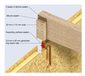
**Figure G.10:** Roof purlin connection TEK system. [43]
