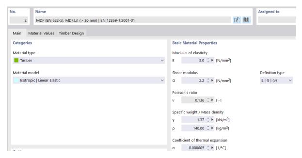
Figure 3.15: Material definition for the core.
