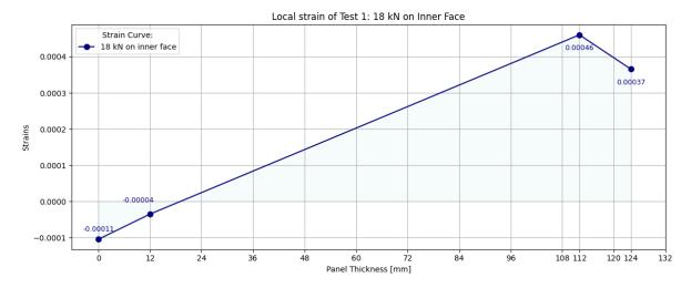
Figure 4.10: Strains of Test 1 inner face loaded with 18 kN.
