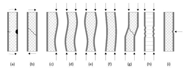
**Figure 2.6:** Sandwich panel failure modes. a) Face yielding/fracture; b) core shear failure; c) face wrinkling - local buckling - delamination; d) face wrinkling - local buckling - delamination; e) face wrinkling - local buckling - delamination; f) general buckling; g) shear crimping; h) face dimpling - only for honeycomb; i) local indentation. [39]
