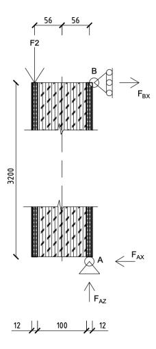
Figure 4.35: Calculation with 6 kN loaded on the outer face
