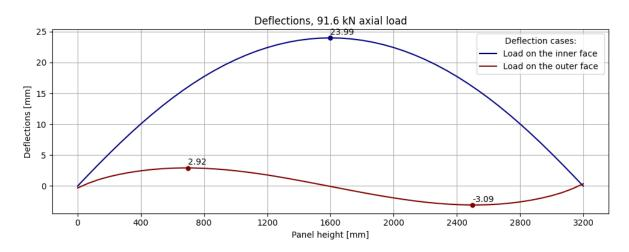
Figure 4.19: Deflections of axial load 91.6 kN.
