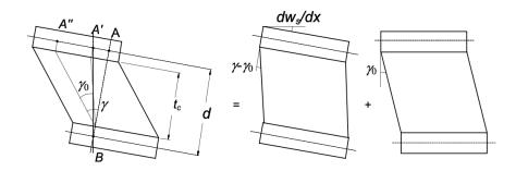
**Figure 2.4:** Shear deformation of a SIP – total deformation; transverse deformations; in-plane deformations
