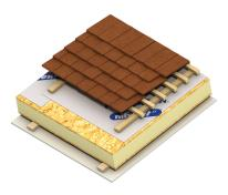
**Figure 1.6:** TEK system roof cladding. [13]
