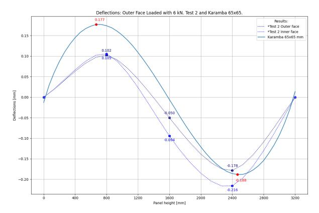
Figure 4.44: Deflections of 6 kN on the outer face - Karamba 65x65 results and test 2.
