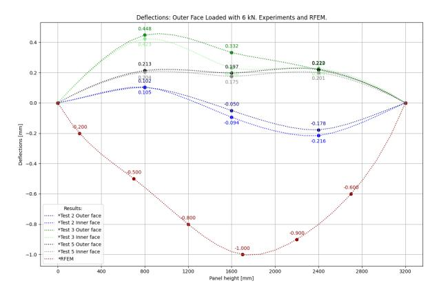
Figure 4.42: Deflections of 6 kN on the outer face - experiments and RFEM.
