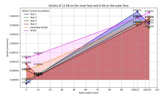
**Figure 4.49:** Strains of 12 kN on the inner face and 6 kN on the outer face (compression is positive and tension is negative).
