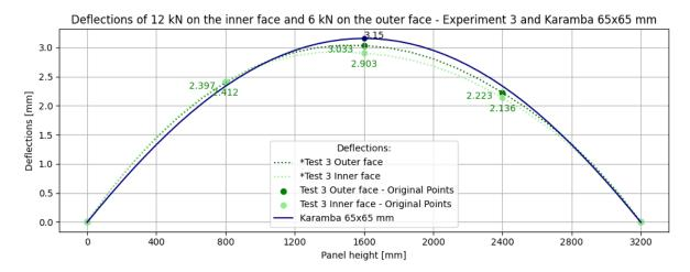
**Figure 4.53:** Experiment 3 and Karamba 65x65 mm deflections of 12 kN on the inner face and 6 kN on the outer face.
