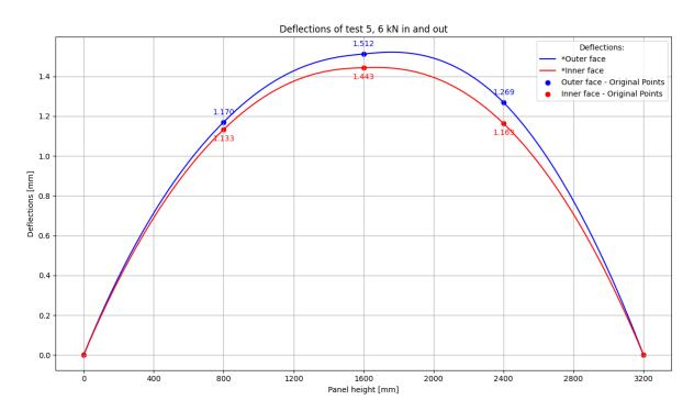
Figure F.31: Test 5 6 kN in and out defl
