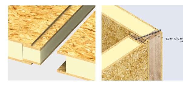
**Figure 2.12:** Wall continuous connection TEK system 1 – mini-SIP connection. [43]
