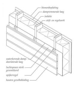
**Figure 1.3:** Timber frame cross-section with timber cladding. [14]
