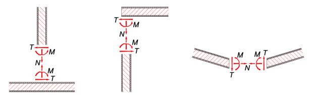
Figure 2.10: Forces acting in the joints [32].
