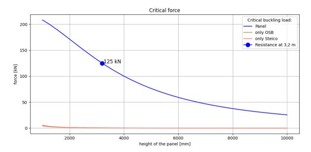
Figure 4.3: Buckling of the panel, and the materials
