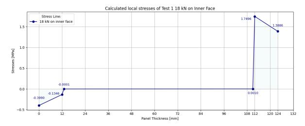
**Figure 4.15:** Stresses of Test 1 inner face loaded with 18 kN.
