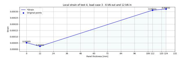
Figure F.26: Test 4 12 kN in and 6 kN out strain - load case 3
