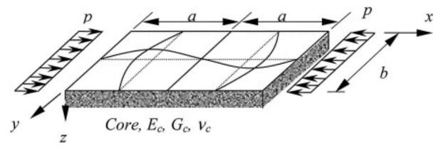
**Figure 2.8:** A plate on elastic foundation buckling shape [40].
