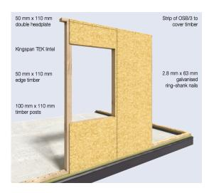
**Figure G.5:** Opening detail TEK system. [43]
