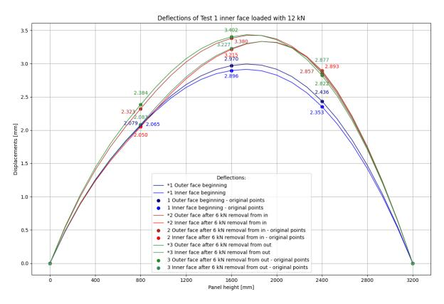
Figure 4.7: Deflections of Test 1 inner face loaded with 12 kN.
