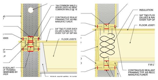
Figure 2.19: Floor beam with a joist hanger [44].
