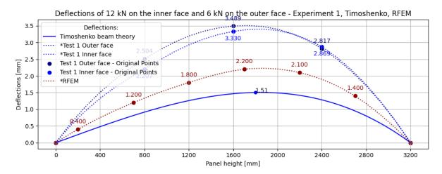
**Figure 4.52:** Experiment 3, Timoshenko and RFEM deflections of 12 kN on the inner face and 6 kN on the outer face.
