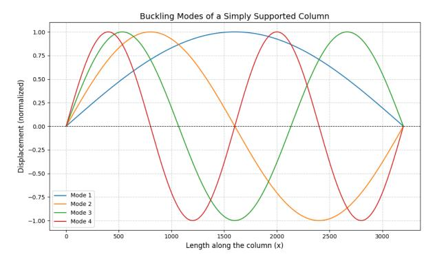
**Figure 4.38:** Buckling modes 1 to 4.
