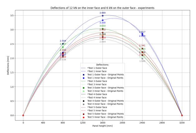
Figure 4.50: Experiments deflections of 12 kN on the inner face and 6 kN on the outer face.
