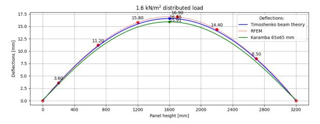
**Figure 4.34:** Deflections of transverse loading under 1.6  $kN/m^2$ .
