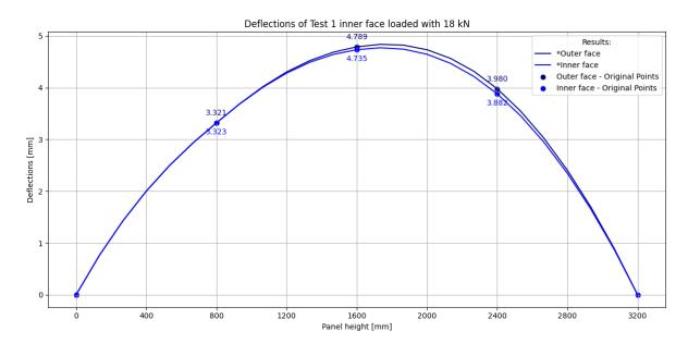
**Figure 4.9:** Deflections of Test 1 inner face loaded with 18 kN.
