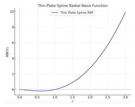
Figure 3.20: Radial basis function of thin plate spline.
