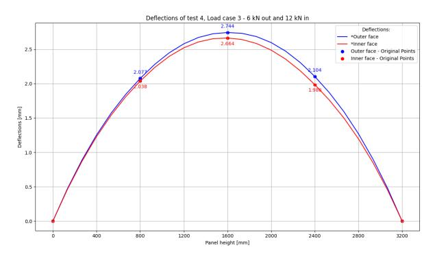
Figure F.25: Test 4 12 kN in and 6 kN out defl - load case 3
