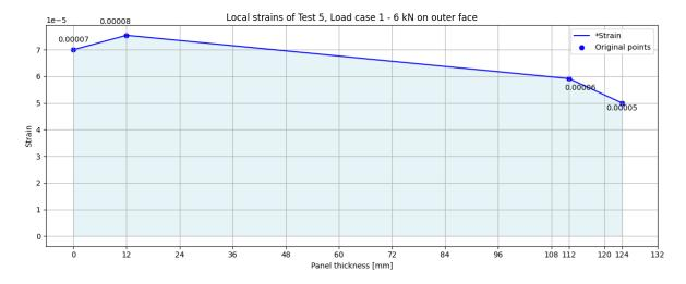
Figure F.34: Test 5 6 kN out strain - load case 1
