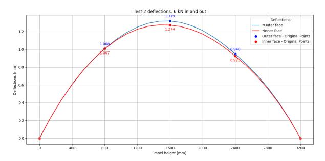
Figure F.7: Test 2 6 kN in and out defl
