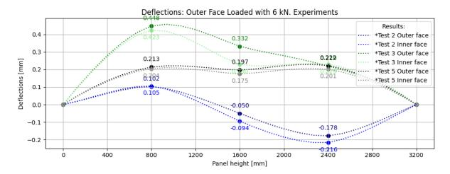
Figure 4.37: Deflections of 6 kN on the outer face experimental results.
