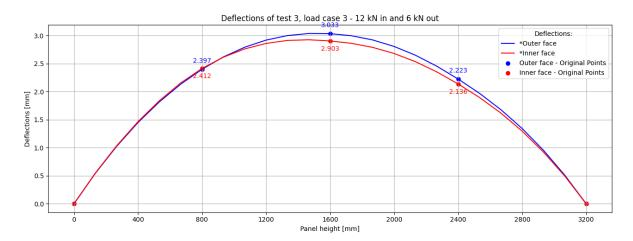
Figure F.17: Test 3 12 kN in and 6 kN out defl - load case 3
