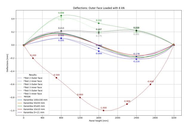
**Figure 4.41:** Deflections of 6 kN on the outer face.
