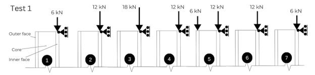
**Figure 4.4:** Loading order of test 1 (also seen in Figure 3.22.
