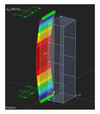
**Figure 4.32:** Karamba3D model under transverse loading.
