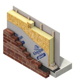
**Figure 1.4:** Kingspan TEK building system with brick cladding. [13]
