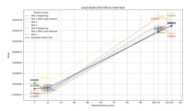
Figure F.4: 6 kN on inner face strains
