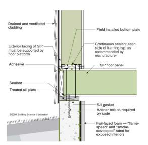
**Figure G.12:** Foundation connection with a floor beam in between. [44]
