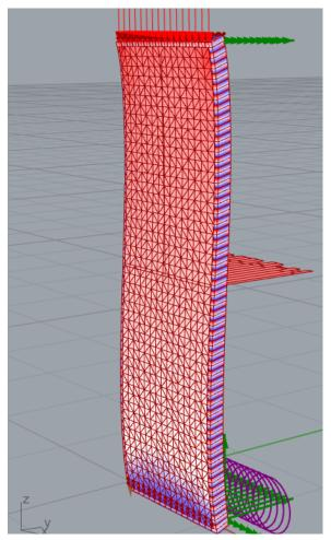
**Figure 4.25:** Outer face loaded deflected Karamba3D model isometric. Red signifies compression and blue signifies tension.
