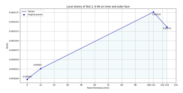
Figure F.8: Test 2 6 kN in and out strain
