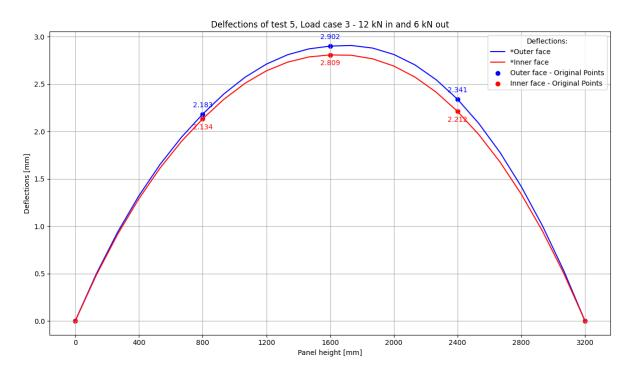
Figure F.35: Test 5 12 kN in and 6 kN out defl - load case 3
