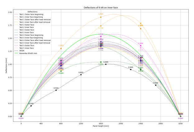
Figure F.3: 6 kN on inner face deflections
