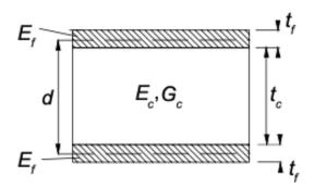
Figure 2.1: Sandwich beam sketch [32].
