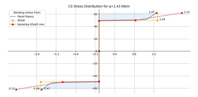
**Figure 4.28:** Cross section bending stress distribution under q=1.43 kN/m.
