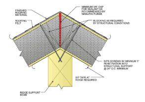
**Figure G.9:** Roof top connection. [44]
