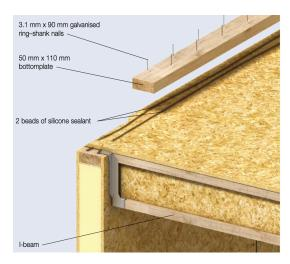
**Figure G.14:** Joist hanger floor connection TEK system 2. [43]
