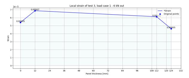
Figure F.20: Test 3 6 kN out strain - load case 1
