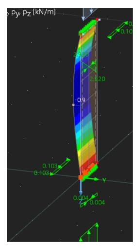
**Figure 4.40:** Outer face loaded RFEM model deformed shape.
