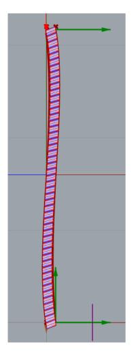
**Figure 4.26:** Outer face loaded deflected Karamba3D model side view. Red signifies compression and blue signifies tension.
