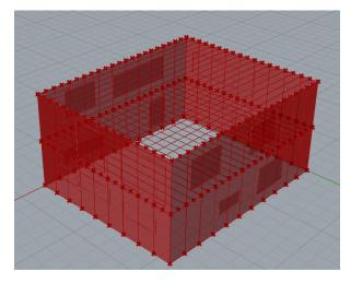
Figure H.8: Grasshopper/Dlubal plug in detailed building for RFEM.
