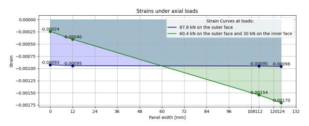
Figure 4.23: Strains of axial load 87.8 kN and 90.4 kN (negative is compression and positive is tension).
