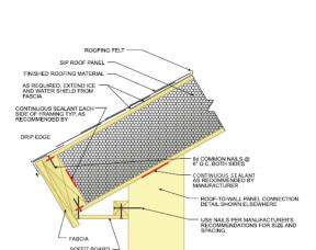
Figure G.6: Roof wall connection 3. [44]
