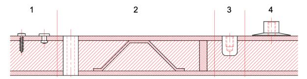
**Figure 2.18:** Connecting insert types – 1) self-tapping, 2) through-thickness, 3) partial, and 4) flared top inserts [32].
