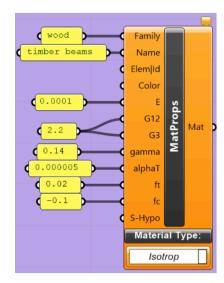
**Figure 3.3:** Predefined Karamba3D material for the beams. E – modulus of elasticity [kN/cm2]; G12 and G3 – shear moduli in different directions [kN/cm2]; gamma – specific weight [kN/m3]; alphaT – heat conductivity [1/C]; ft – tensile strength [kN/cm2]; fc – compressive strength [kN/cm2]
