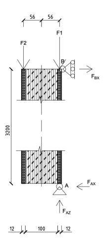
Figure 4.46: Loading on the inner and outer face.
