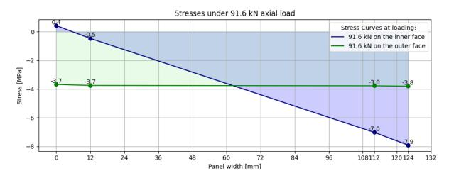
Figure 4.20: Stresses of axial load 91.6 kN (negative is compression and positive is tension).
