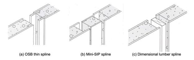
**Figure 2.11:** Panel to panel connection types [42].
