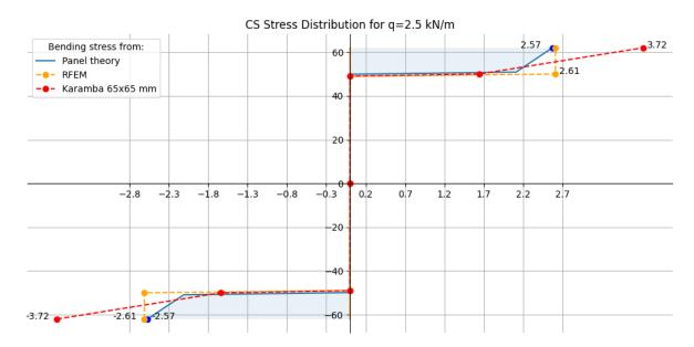
Figure 4.29: Cross section bending stress distribution under q=2.5 kN/m.
