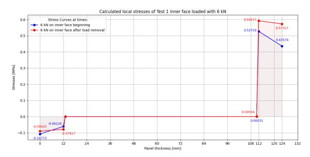
**Figure 4.13:** Calculated stresses of Test 1 inner face loaded with 6 kN.
