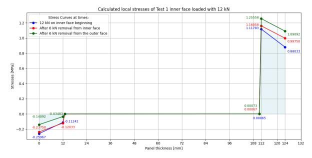
Figure 4.14: Stresses of Test 1 inner face loaded with 12 kN.
