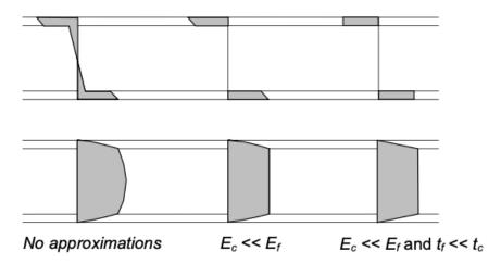
Figure 2.3: Direct and shear stresses. Two approximations. [32]
