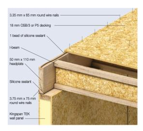
**Figure G.16:** Rim board floor connection TEK system 1. [43]
