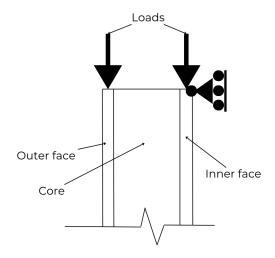
Figure 3.5: Loading schema.
