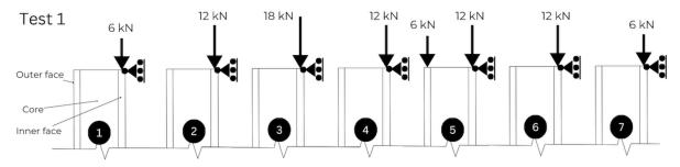
Figure 3.22: Tests loading order.
