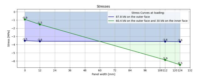
Figure 4.22: Stresses of axial load 87.8 kN and 90.4 kN (negative is compression and positive is tension).
