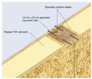
Figure 2.14: Wall continuous connection TEK system Figure 2.15: Wall continuous connection TEK system 2 – thin spline connection [43].
