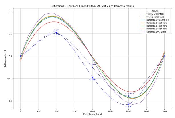
Figure 4.43: Deflections of 6 kN on the outer face - Karamba results and test 2.
