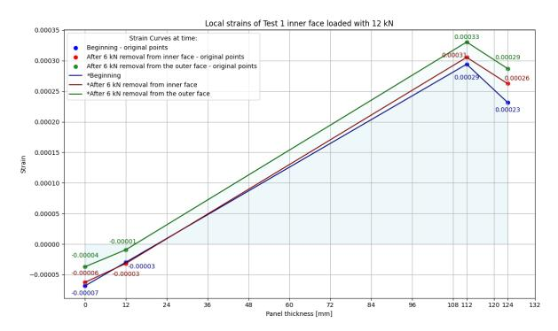
Figure 4.8: Strains of Test 1 inner face loaded with 12 kN.
