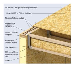
**Figure G.15:** Joist hanger floor connection TEK system 1. [43]
