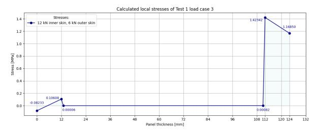
Figure 4.16: Stresses of Test 1 inner face loaded with 12 kN and outer face loaded with 6 kN.
