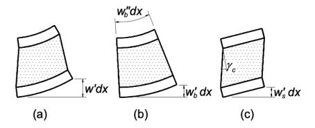
Figure 2.5: SIP deformations: a) total deformation; b) bending deformation; c) shear deformation [32].
