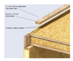
**Figure G.17:** Rim board floor connection TEK system 2. [43]
