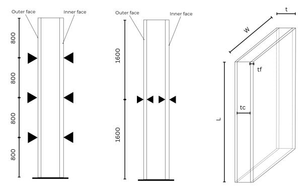
**Figure 3.17:** a) Horisontal deflection measurements locations; b) Local strains measurements locations; c) Panel sketch.
