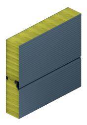
**Figure 1.1:** Sandwich panel with metal skins and mineral wool insulation. [12]
