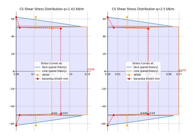
**Figure 4.30:** Cross section shear stress distribution for **Figure 4.31:** Cross section shear stress distribution for q=1.43 kN/m.
