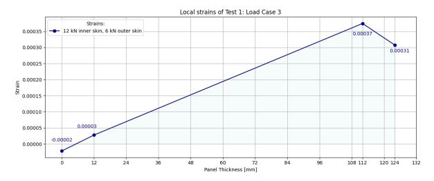
Figure 4.12: Strains of Test 1 inner face loaded with 12 kN and outer face loaded with 6 kN.
