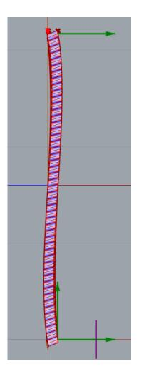
**Figure 4.39:** Outer face loaded Karamba3D model deformed shape.
