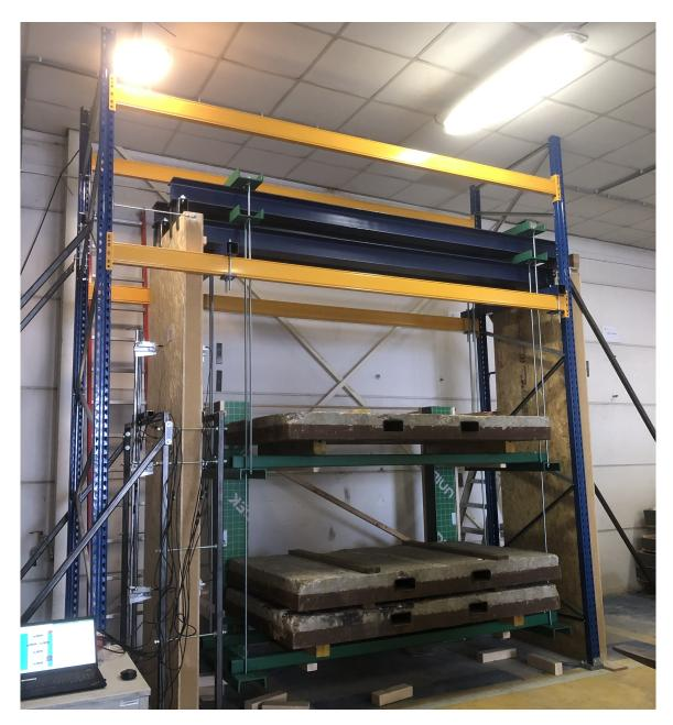
Figure 3.21: Test rig set up - load case 3 - 12 kN on the inner face, 6 kN on the outer face.
