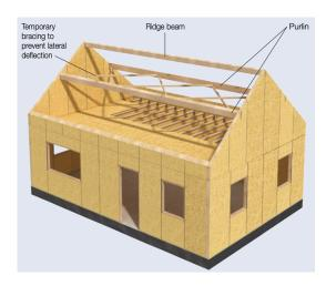
Figure G.11: Roof beams TEK system. [43]
