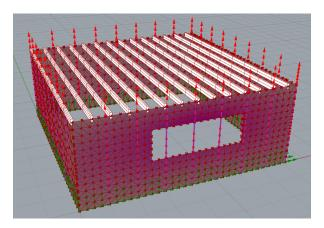
**Figure H.5:** Karamba simple building with joints and support conditions 2.
