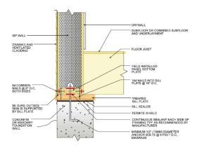
**Figure G.13:** Foundation connection directly on the foundation. [44]
