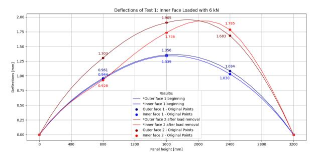
**Figure 4.5:** Deflections of Test 1 inner face loaded with 6 kN.
