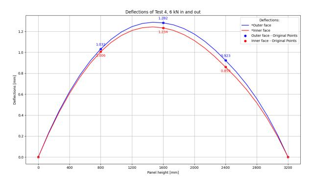
Figure F.23: Test 4 6 kN in and out defl
