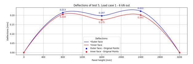
Figure F.33: Test 5 6 kN out defl - load case 1
