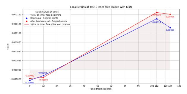
Figure 4.6: Strains of Test 1 inner face loaded with 6 kN.
