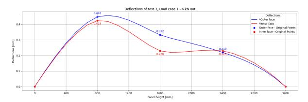
Figure F.19: Test 3 6 kN out defl - load case 1
