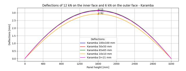
Figure 4.51: Karamba deflections of 12 kN on the inner face and 6 kN on the outer face.
