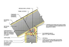
Figure G.4: Roof wall connection 2. [44]
