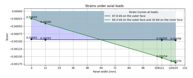
Figure 4.24: Strains of axial load 87.8 kN and 90.4 kN (negative is compression and positive is tension).
