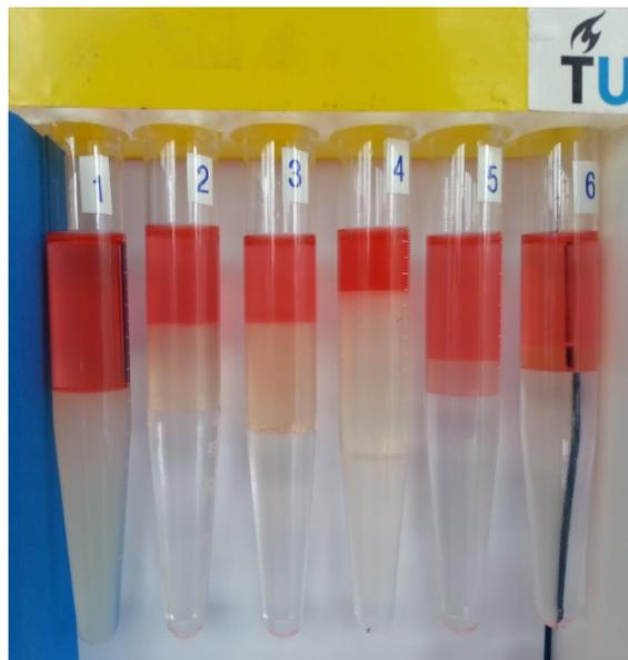
**Fig. 4.1:** Phase behaviour of IOS and n-hexadecane with the glass tube salinity scan method. Salinity (NaCl) varies from left to right 1.0 to 6.0 weight per cent in the surfactant solution.
