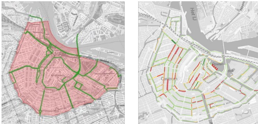
Figure 4.2: Weight restriction zone and state of the Amsterdam canal walls (Retrieved from: (Lof & Olsthoorn, 2019))
