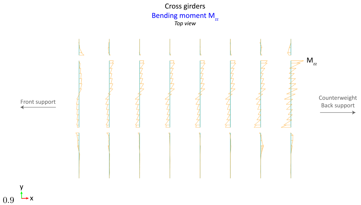
Figure G.49: Cross girders - vertical load case - bending around local z- axis
