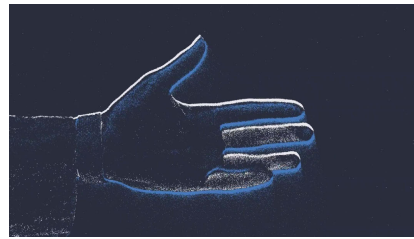
(b) An event camera captures which pixels have changed in intensity.
