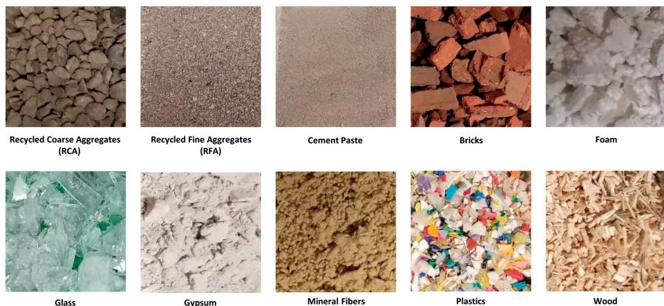
Figure 5.2: Demolition waste samples
