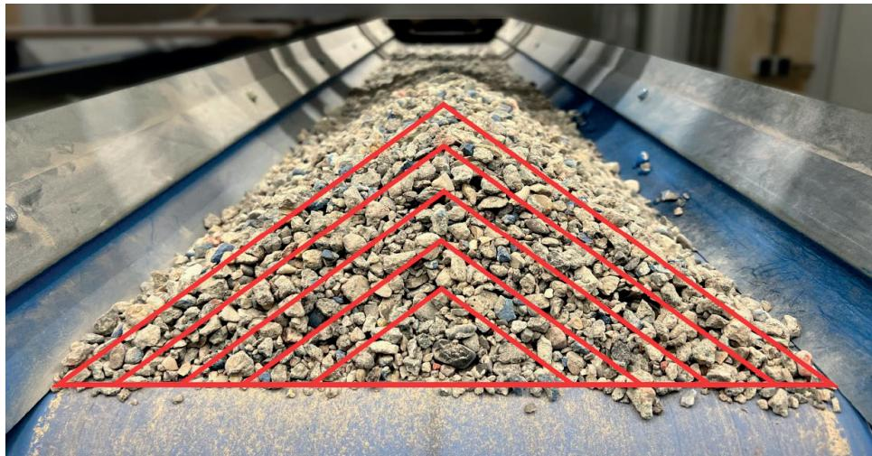
Figure 2.6: Layered formation of RCA piles
