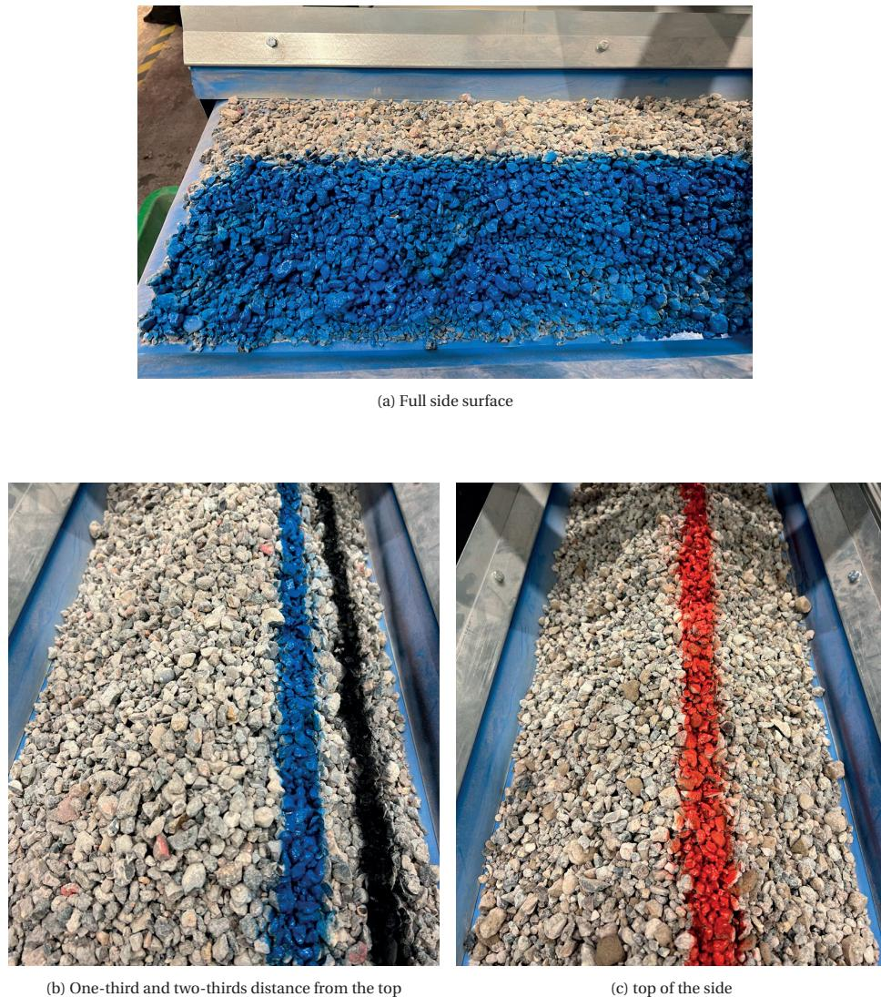
Figure 4.6: Sampling from the side surface of the RCA piles
