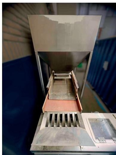
(a) Conical feeder and splitter
